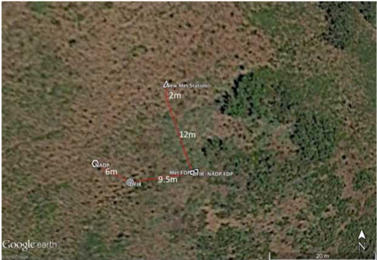
Figure 3 Layout of Met Station, DFIR and Wet Deposition Collector with Associated Field Device Posts.
