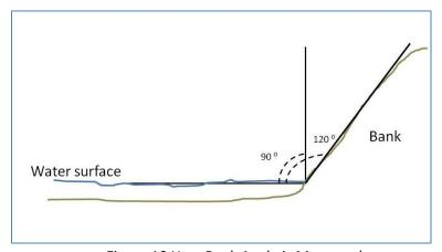
Figure 10 How Bank Angle is Measured
