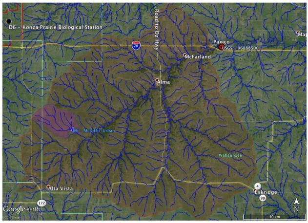
Figure 34 Map showing location of the USGS gauging station 06888500 at Paxico and the relative catchment size of Mill Creek (Orange) compared to McDiffett (Purple).
