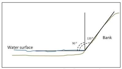
Figure 26 How Bank Angle is Measured
