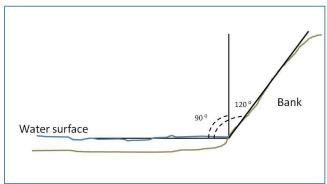
Figure 61 How Bank Angle is Measured
