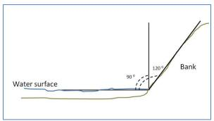
Figure 46 How Bank Angle is Measured
