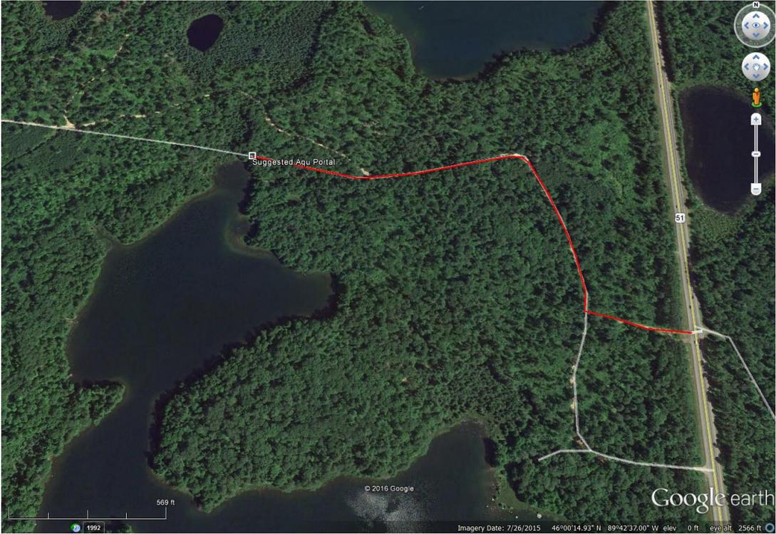
**Figure 27** The suggested power run at D05 Little Rock Lake, shown in red.
