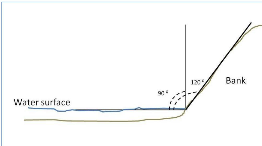
**Figure 41 How Bank Angle is Measured**
