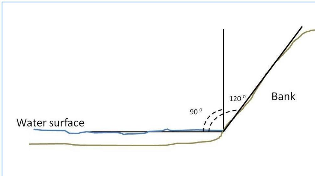
**Figure 18 How Bank Angle is Measured**
