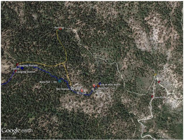
Figure 22 Map of site location showing the access roads (white) and pathways (yellow), location of the access gate and parking area.
