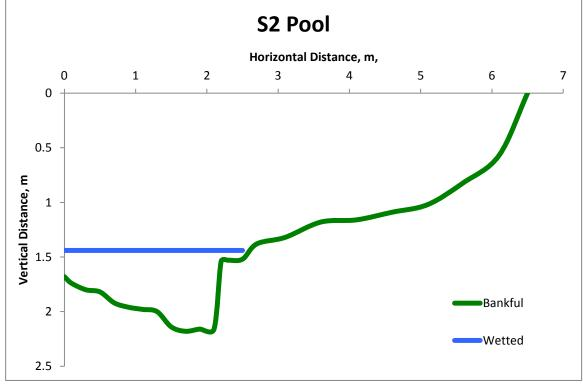
Figure 20 Cross sectional geomorphology survey of S2 pool.
