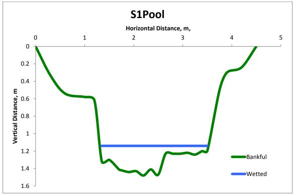
Figure 19 Cross sectional geomorphology survey of S1 pool.
