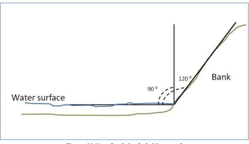
Figure 41 How Bank Angle is Measured
