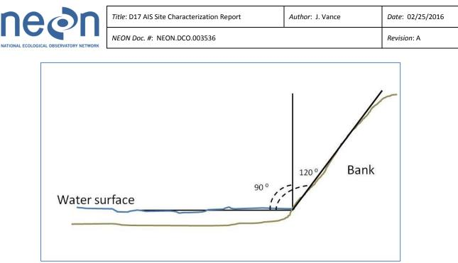
Figure 18 How Bank Angle is Measured
