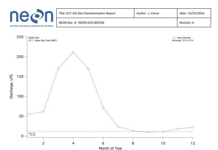
Figure 30 Hydrograph of mean monthly discharge based on historic data and catchment scaling.
