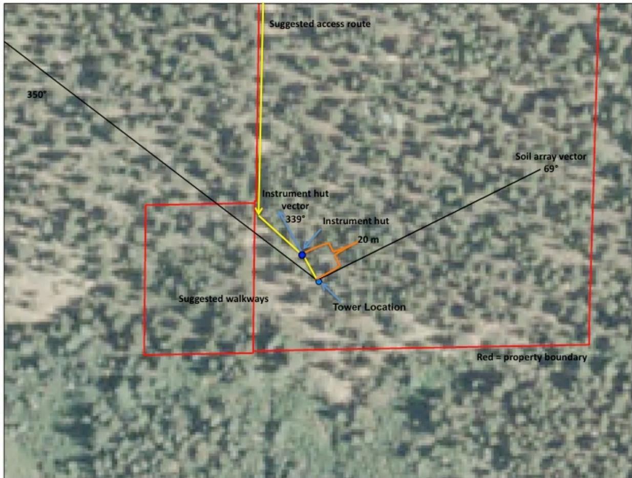
**Figure 6.** Plan view of the CASTNET Relocatable site location
