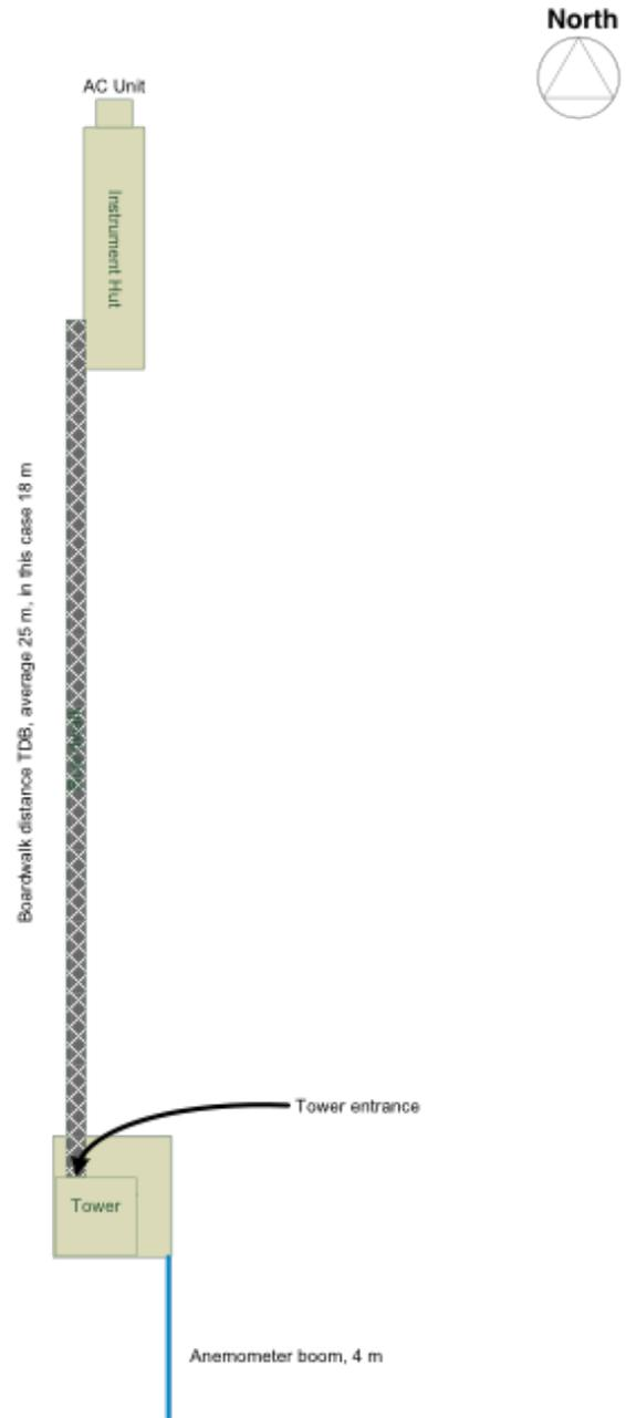
**Figure 8.** Generic plan view of the tower, Instrument hut and boardwalk pathways
