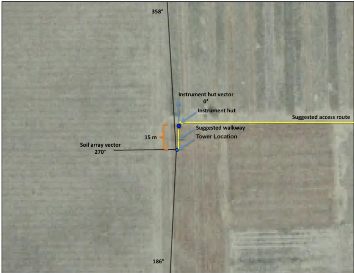
**Figure 4.** Plan view of the North Sterling Relocatable site location
