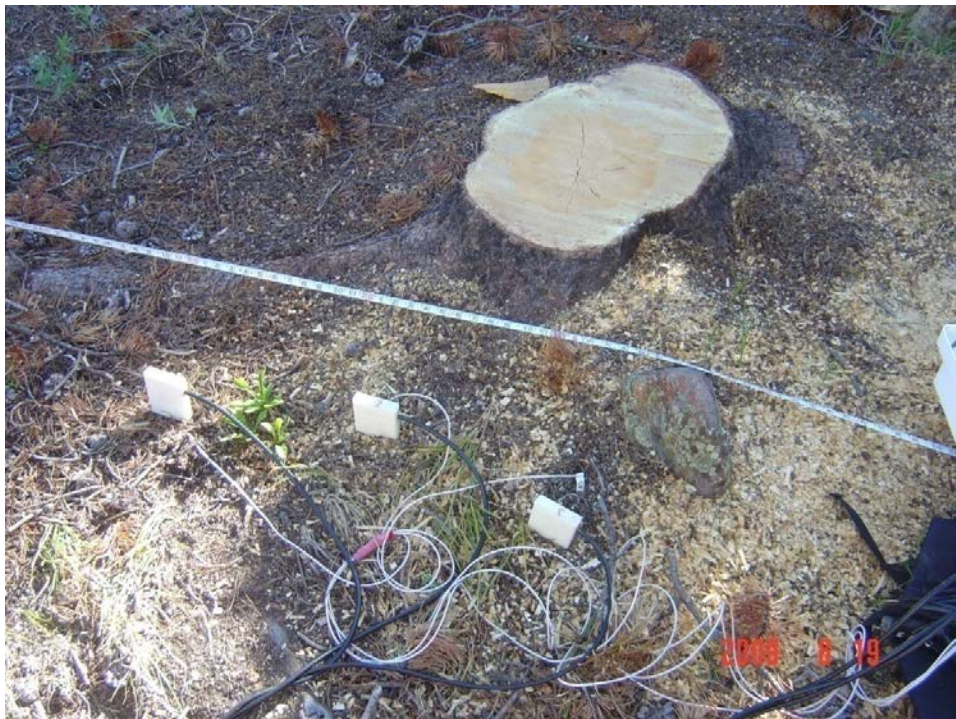
Figure 49. Three replicates of soil temperature and SWC were measured at each sampling point at fixed-depth (0-20 cm).
