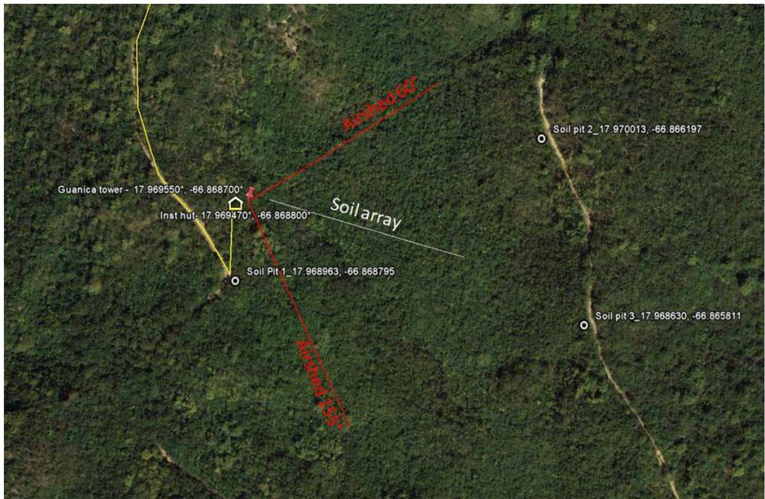
Figure 9. Site layout at Guanica to show soil array
