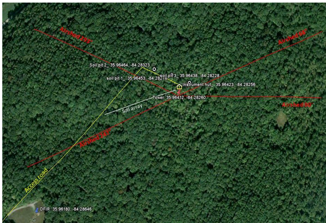
Figure 12. Site layout at ORNL Walker Branch Advanced tower site showing soil array and location of the FIU soil pit.
