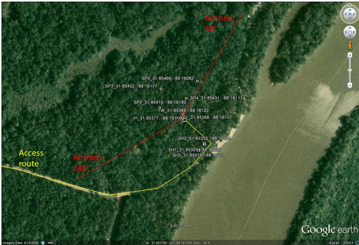
Figure 27. Site layout at Lenoir Landing showing soil array and location of the FIU soil pit.
