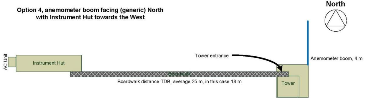
**Figure 53.** Generic diagram to demonstration the relationship between tower and instrument hut when boom facing north and instrument hut on the west towards the tower.
