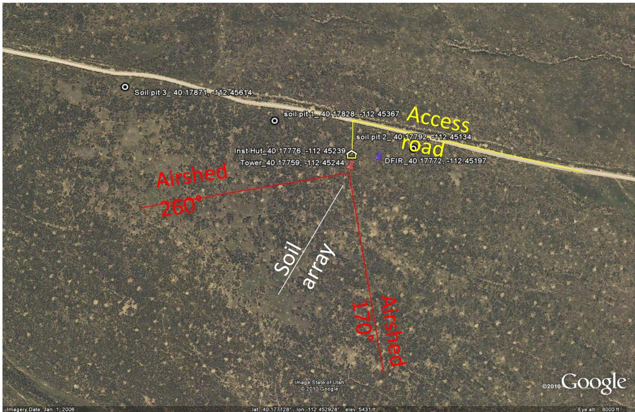
Figure 11. Site layout at Onaqui-Ault Advance site showing soil array and location of the FIU soil pits.
