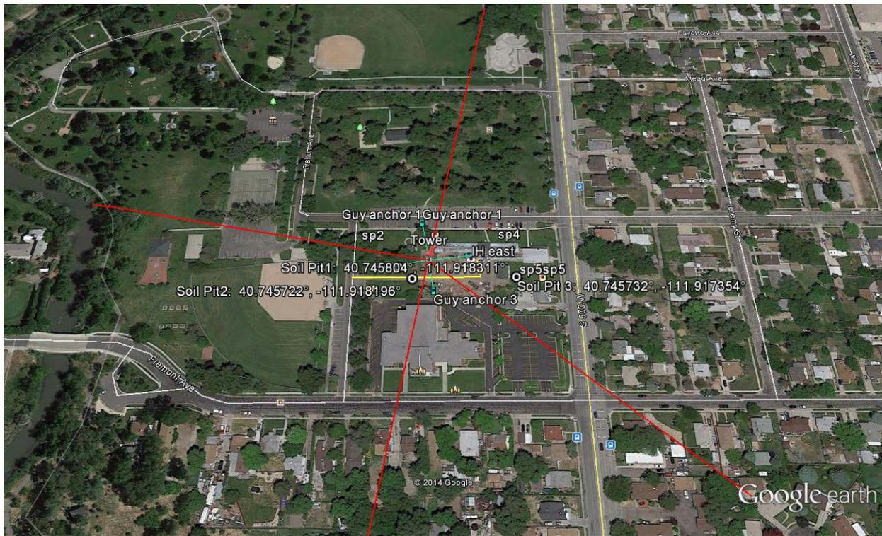
Figure 25. Site layout at SLC urban showing soil array and location of the FIU soil pit.
