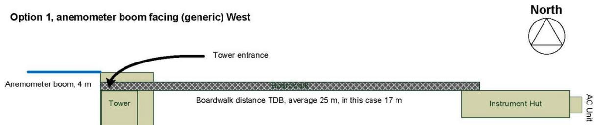
**Figure 34.** Generic diagram to demonstration the relationship between tower and instrument hut when boom facing west and instrument hut on the east towards the tower.
