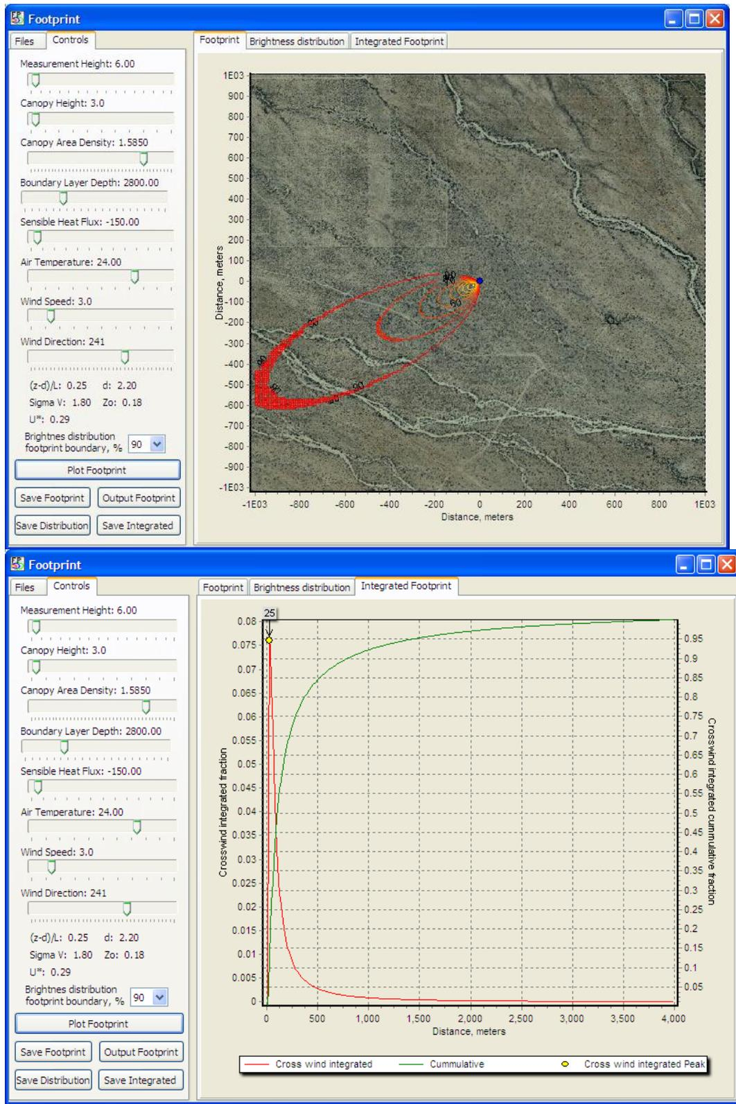
Figure 15. SRER summer nighttime (stable) footprint output with mean wind speed.
