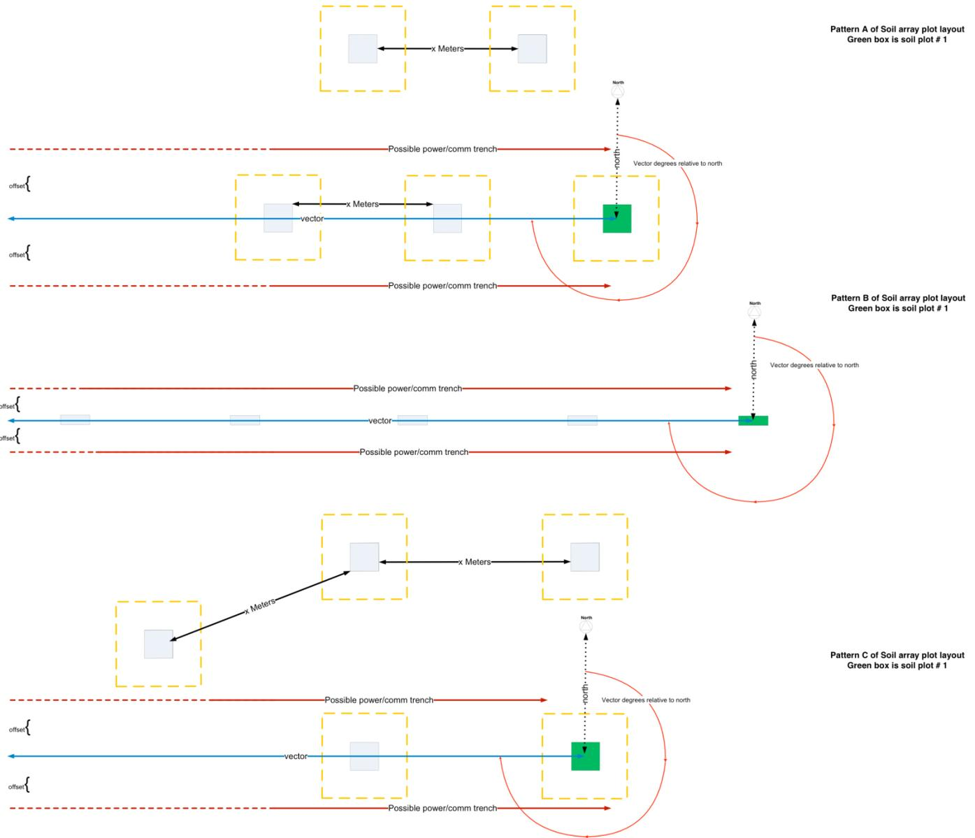
**Figure A1.** Conceptual diagram of Soil Array Patterns
