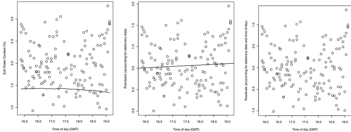
**Figure 29.** Left graph: mobile (circles) and stationary (line) soil water content data. Center graph: water content data after correcting for changes in water content in the stationary data (circles) and a linear regression based on time of day (line). Right graph: residual water content data after correcting for changes water content in the stationary data and the time of day regression. Data in the right graph were used for the semivariogram analysis.
