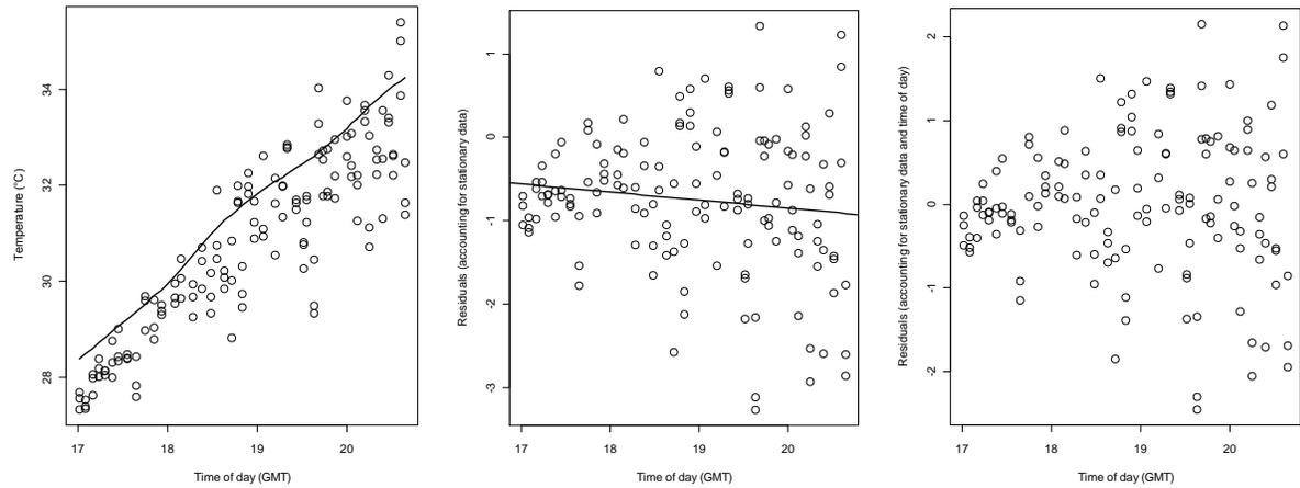
**Figure 7.** Left graph: mobile (circles) and stationary (line) soil temperature data. Center graph: temperature data after correcting for changes in temperature in the stationary data (circles) and a linear regression based on time of day (line). Right graph: residual temperature data after correcting for changes temperature in the stationary data and the time of day regression. Data in the right graph were used for the semivariogram analysis.
