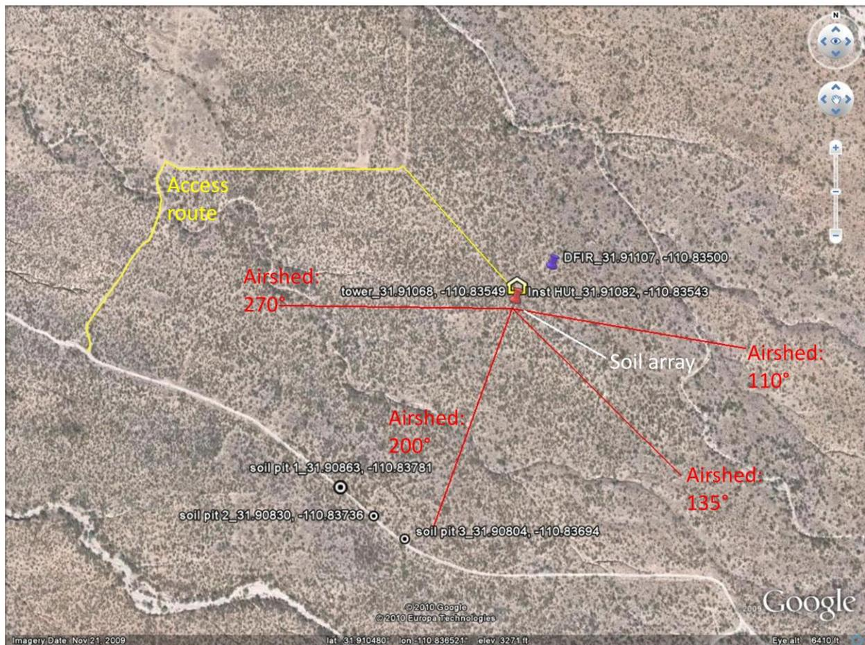
**Figure 11.** Site layout at Santa Rita showing soil array and location of the FIU soil pit.
