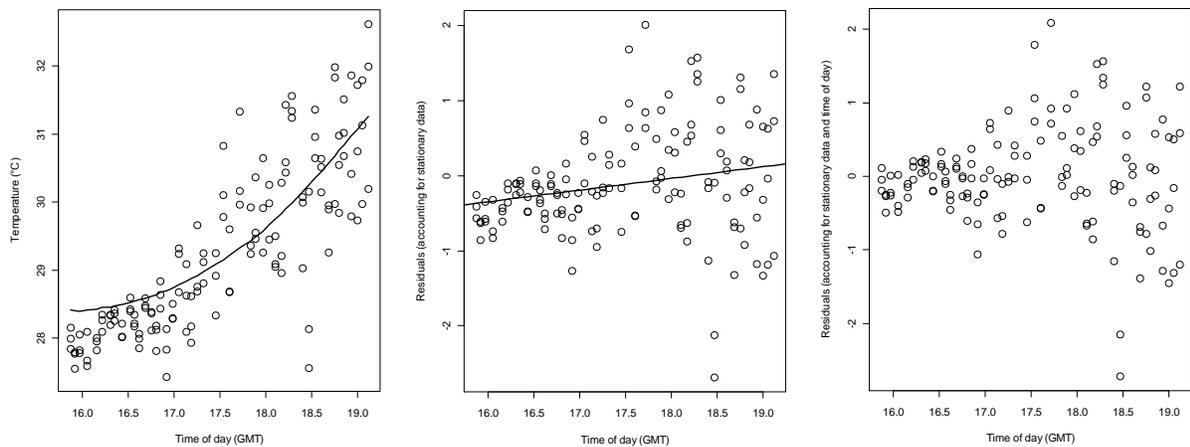
**Figure 27.** Left graph: mobile (circles) and stationary (line) soil temperature data. Center graph: temperature data after correcting for changes in temperature in the stationary data (circles) and a linear regression based on time of day (line). Right graph: residual temperature data after correcting for changes temperature in the stationary data and the time of day regression. Data in the right graph were used for the semivariogram analysis.
