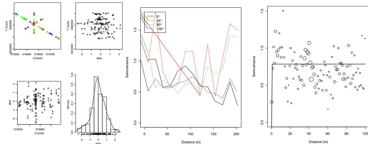
**Figure 8.** Left graphs: exploratory data analysis plots for residuals of temperature. Center graph: directional semivariograms for residuals of temperature. Right graph: empirical semivariogram (circles) and model (line) fit to residuals of temperature.
