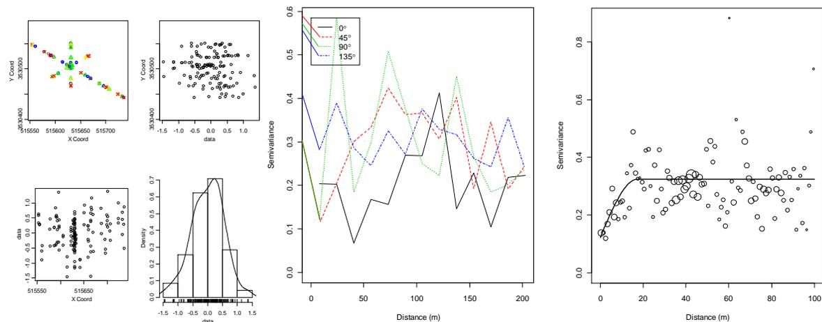
**Figure 10.** Left graphs: exploratory data analysis plots for residuals of soil water content. Center graph: directional semivariograms for residuals of water content. Right graph: empirical semivariogram (circles) and model (line) fit to residuals of water content.
