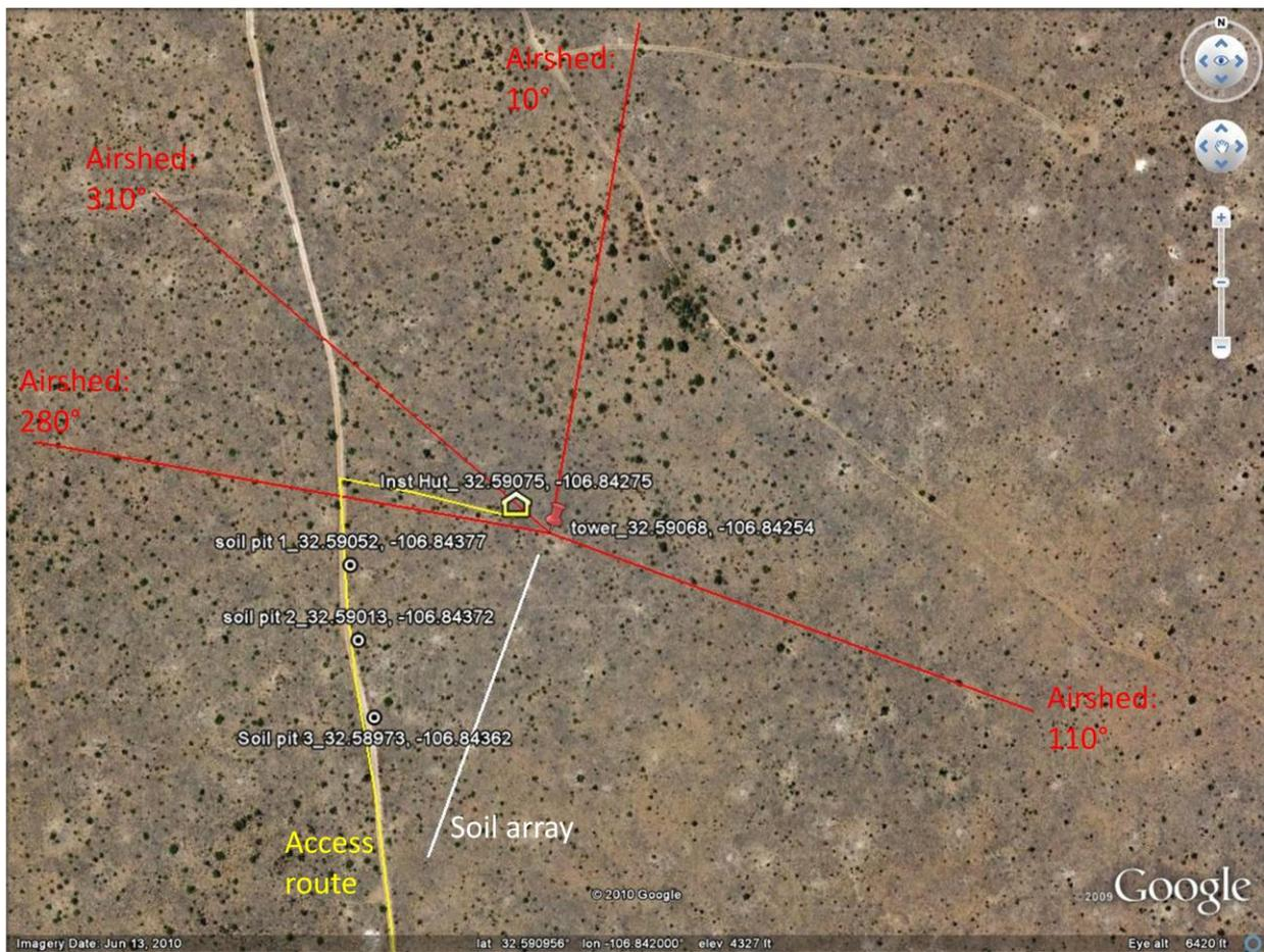
**Figure 31.** Site layout at Jornada relocatable site showing soil array and location of the FIU soil pit.
