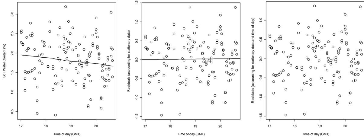
**Figure 9.** Left graph: mobile (circles) and stationary (line) soil water content data. Center graph: water content data after correcting for changes in water content in the stationary data (circles) and a linear regression based on time of day (line). Right graph: residual water content data after correcting for changes water content in the stationary data and the time of day regression. Data in the right graph were used for the semivariogram analysis.
