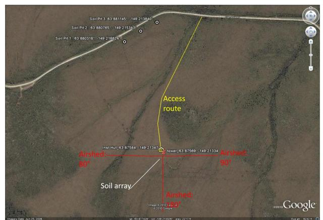
Figure 74. Site layout at Eight Mile showing soil array and location of the FIU soil pit.
