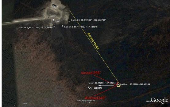
Figure 54. Site layout at Poker Flats Relocatable showing soil array and location of the FIU soil pit.
