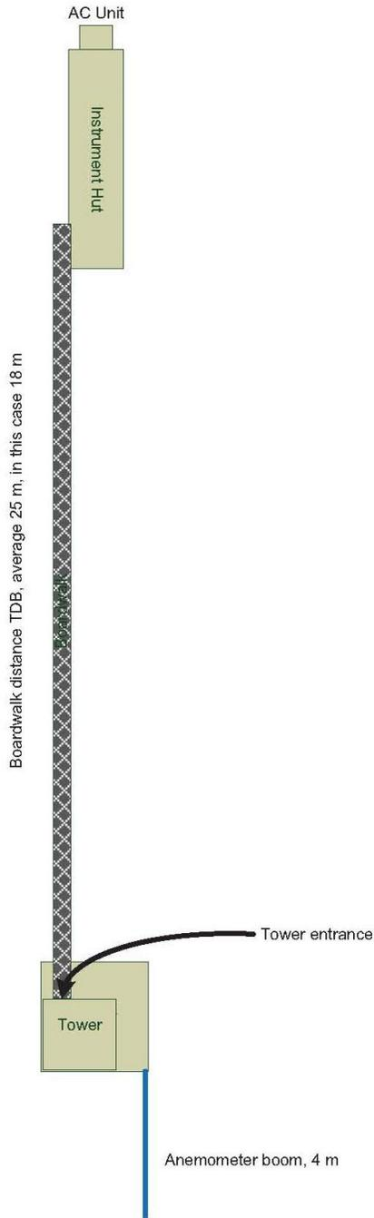
**Figure 1** Generic diagram to demonstration the relationship between tower and instrument hut when boom facing south and instrument hut on the north towards the tower.
