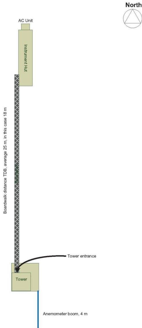
**Figure 8.** Generic diagram to demonstration the relationship between tower and instrument hut when boom facing south and instrument hut on the north towards the tower.
