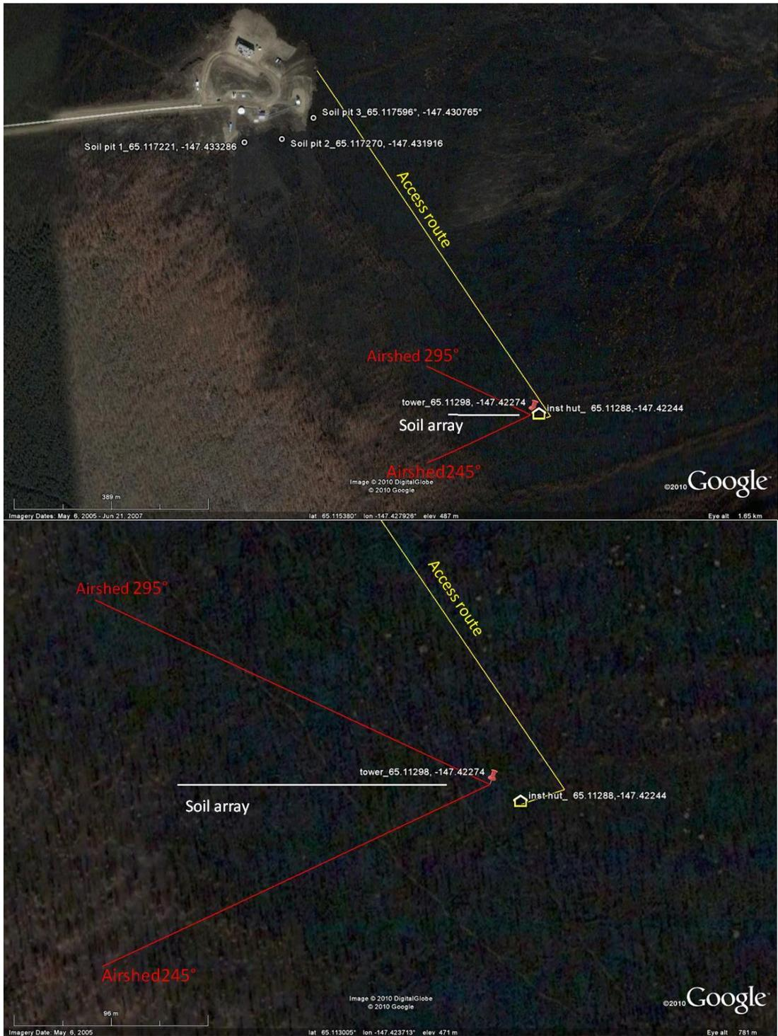
**Figure 7.** Site layout for Caribou Poker Relocatable site. Top panel shows the general site layout. Lower panel shows detailed information for tower, instrument hut, soil array and access boardwalk. i) new tower location is presented (red pin), ii) red lines indicate the airshed boundaries. Vectors from 245° to 295° (major airshed, clockwise from 245°) would have
