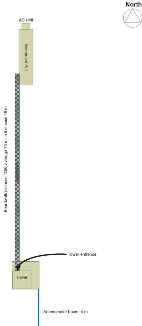
**Figure 4.** Generic diagram to demonstration the relationship between tower and instrument hut when boom facing south and instrument hut on the north towards the tower.
