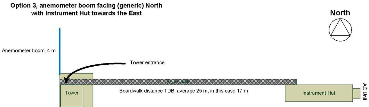
**Figure 6.** Generic diagram to demonstration the relationship between tower and instrument hut when boom facing north and instrument hut on the south towards the tower.
