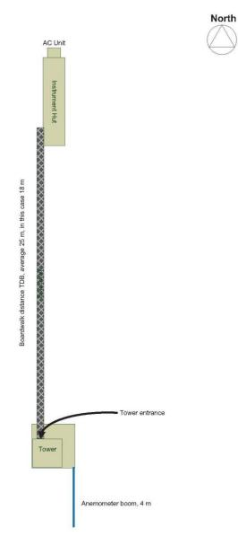
**Figure 8.** Generic diagram to demonstration the relationship between tower and instrument hut when boom facing south and instrument hut on the north towards the tower.
