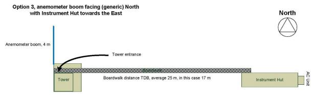
**Figure 6.** Generic diagram to demonstration the relationship between tower and instrument hut when boom facing north and instrument hut on the south towards the tower.
