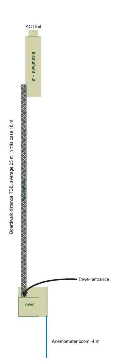
**Figure 1** Generic diagram to demonstration the relationship between tower and instrument hut when boom facing south and instrument hut on the north towards the tower.
