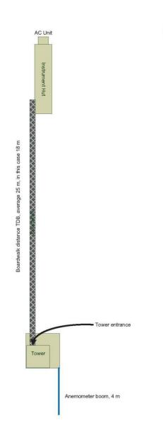
**Figure 4.** Generic diagram to demonstration the relationship between tower and instrument hut when boom facing south and instrument hut on the north towards the tower.
