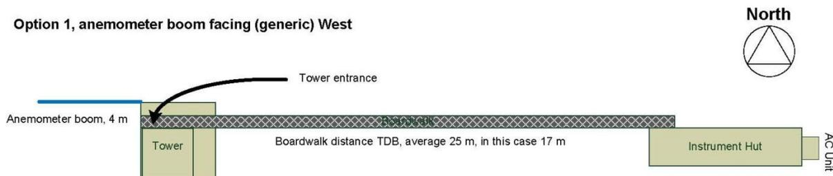
**Figure 40** Generic diagram to demonstration the relationship between tower and instrument hut when boom facing west and instrument hut on the east towards the tower.
