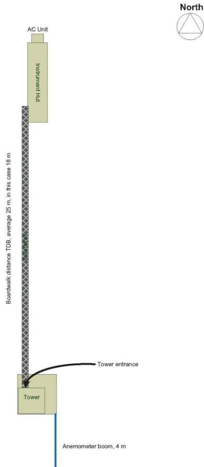
**Figure 60.** Generic diagram to demonstration the relationship between tower and instrument hut when boom facing south and instrument hut on the north towards the tower.
