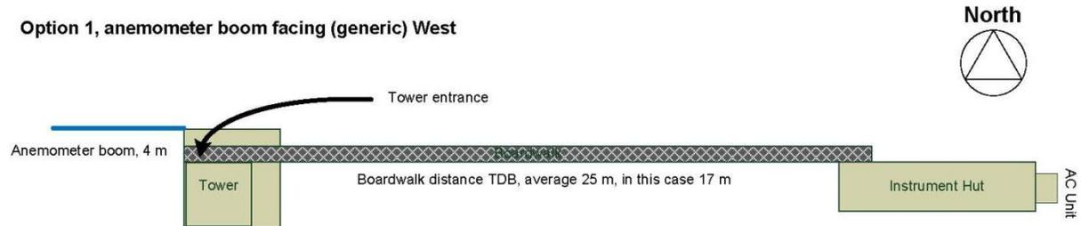
**Figure 21.** Generic diagram to demonstration the relationship between tower and instrument hut when boom facing west and instrument hut on the east towards the tower.
