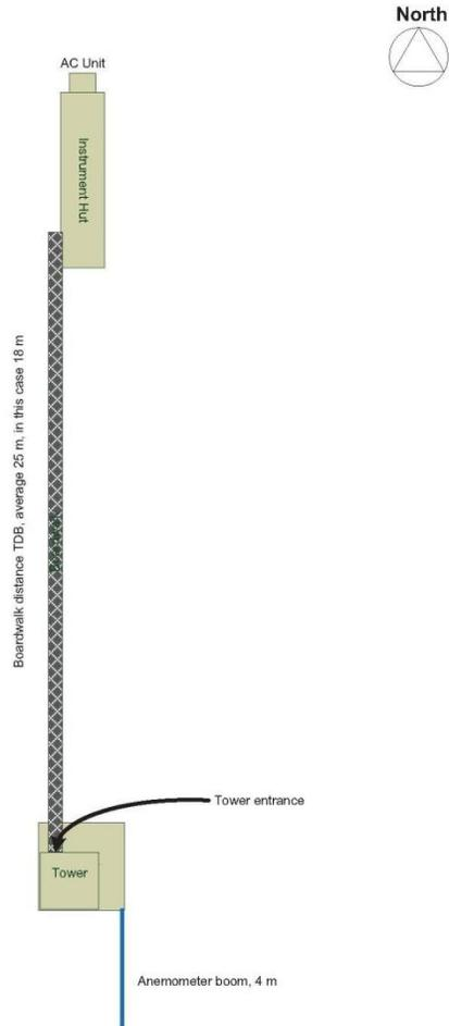
**Figure 5.** Generic diagram to demonstration the relationship between tower and instrument hut when boom facing south and instrument hut on the north towards the tower.
