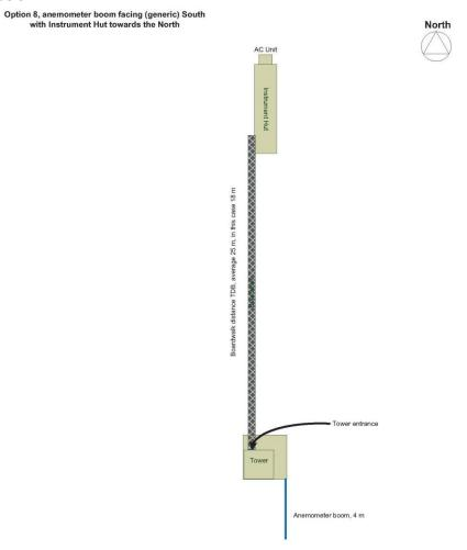
**Figure 5.** Generic diagram to demonstration the relationship between tower and instrument hut when boom facing south and instrument hut on the north towards the tower.
