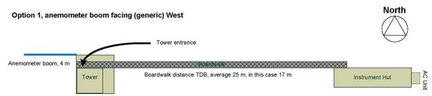
**Figure 1.** Generic diagram to demonstration the relationship between tower and instrument hut when boom facing west and instrument hut on the east towards the tower.
