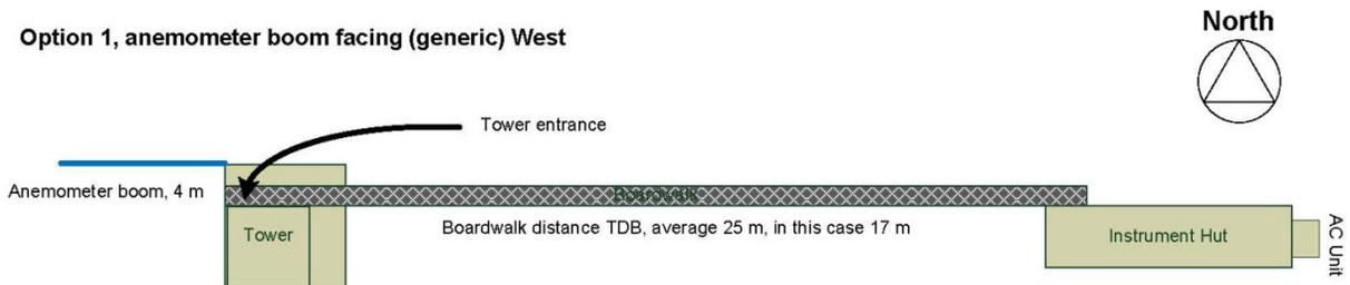
**Figure 63.** Generic diagram to demonstration the relationship between tower and instrument hut when boom facing west and instrument hut on the east towards the tower.
