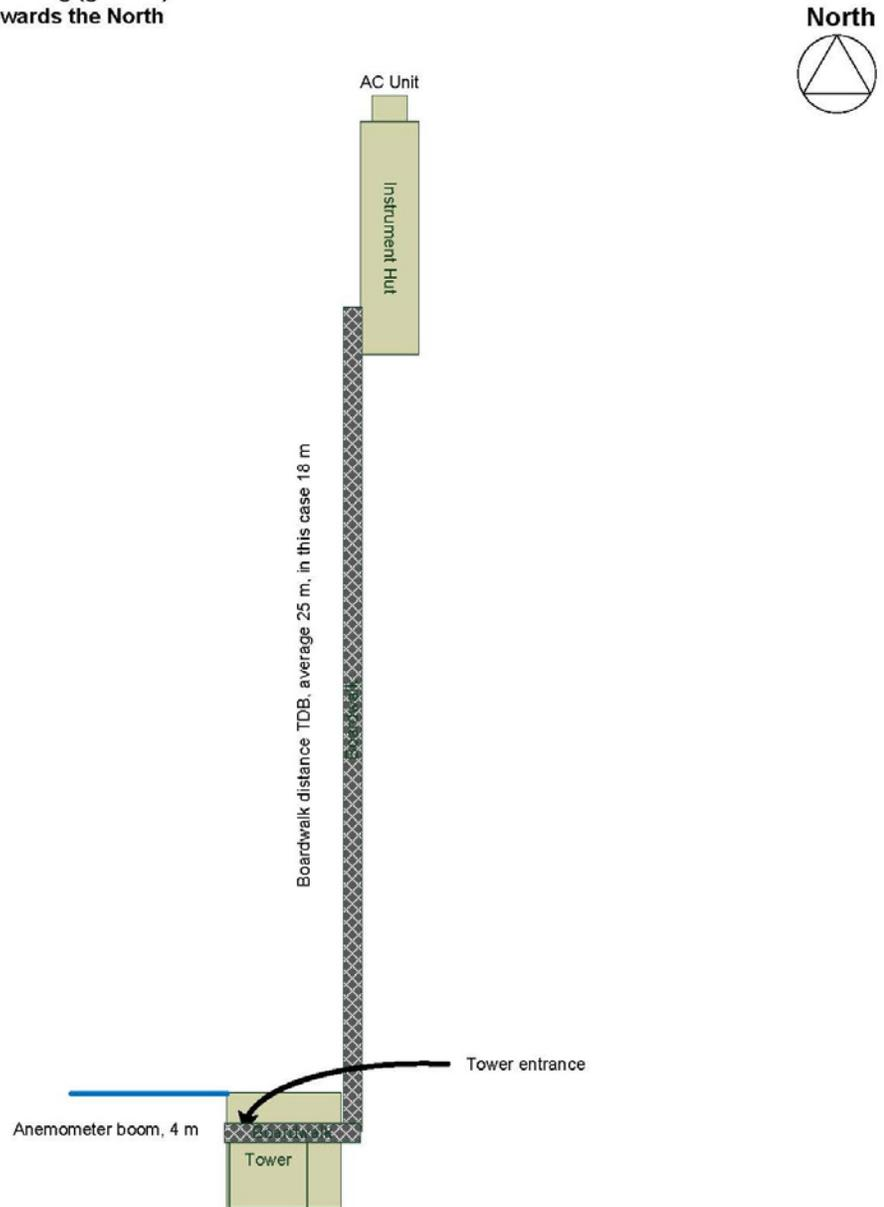
**Figure 40.** Generic diagram to demonstration the relationship between tower and instrument hut when boom facing west and instrument hut on the north towards the tower.
