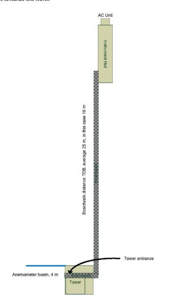
**Figure 40.** Generic diagram to demonstration the relationship between tower and instrument hut when boom facing west and instrument hut on the north towards the tower.
