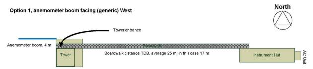
**Figure 19**. Generic diagram to demonstration the relationship between tower and instrument hut when boom facing south and instrument hut on the east towards the tower.
