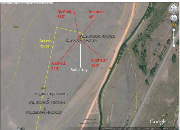
Figure 53. Site layout at Paradise Valley showing soil array and location of the FIU soil pit.
