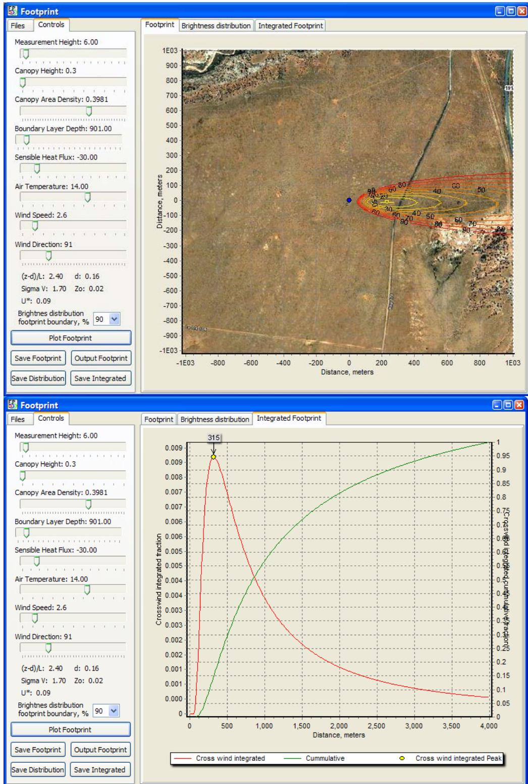
Figure 38. Moab Relocatable site winter nighttime (stable) footprint output with mean wind speed.
