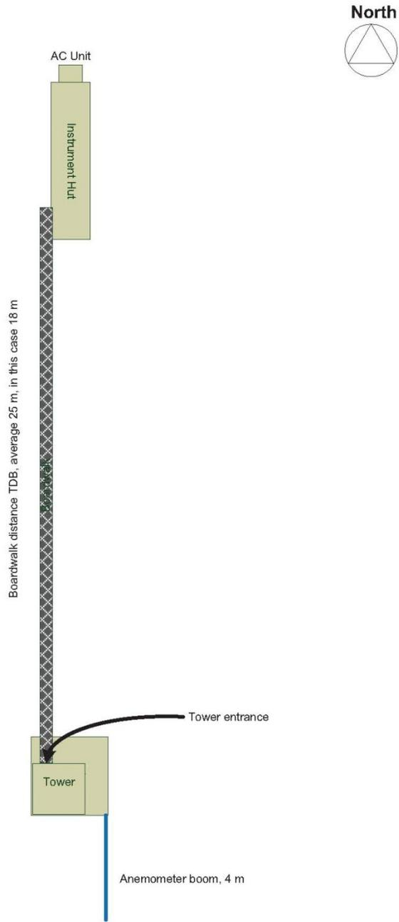
**Figure 40.** Generic diagram to demonstration the relationship between tower and instrument hut when boom facing south and instrument hut on the north towards the tower.
