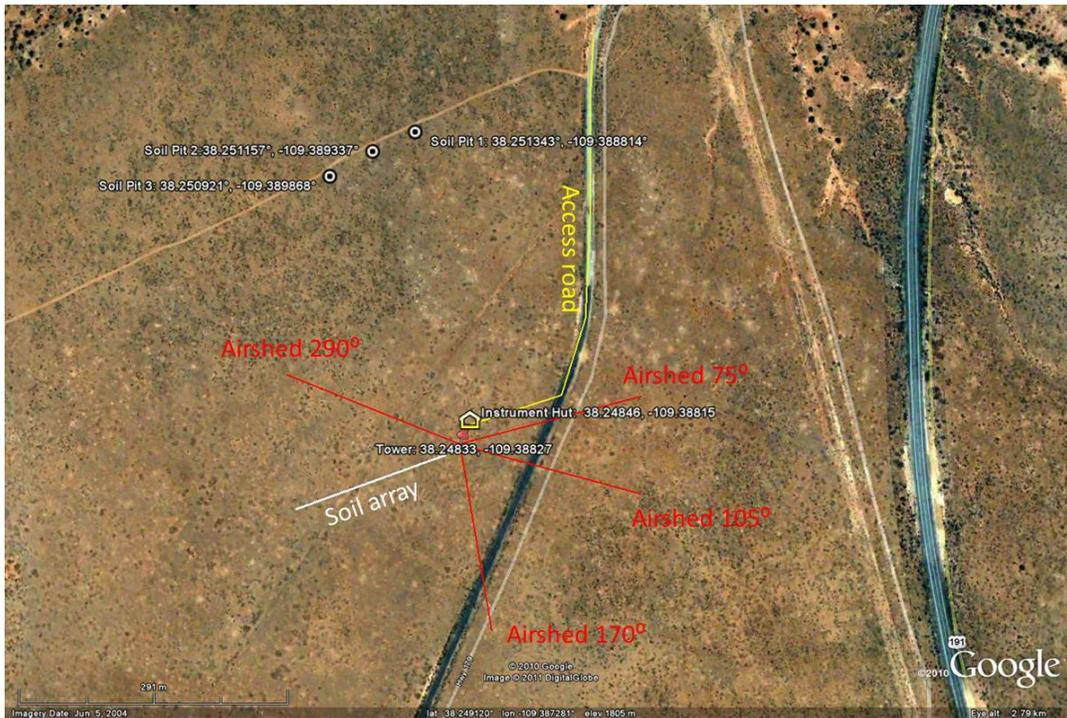
**Figure 31.** Site layout at Moab showing soil array and location of the FIU soil pits.
