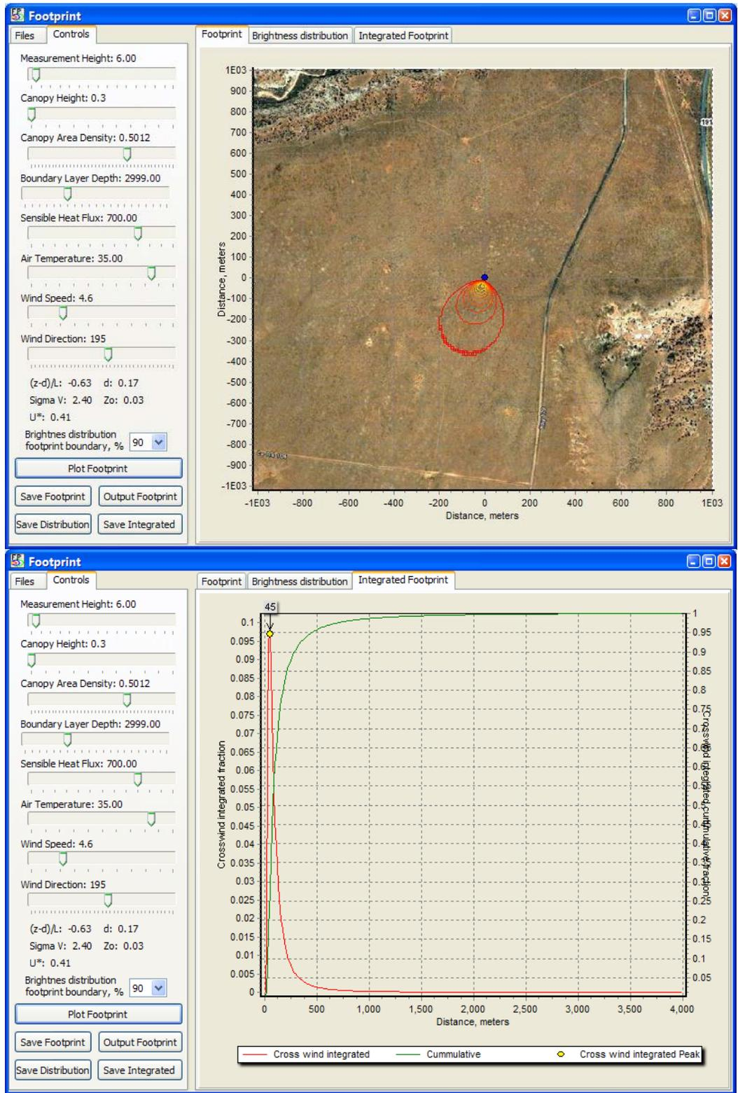
Figure 34. Moab Relocatable site summer daytime (convective) footprint output with mean wind speed
