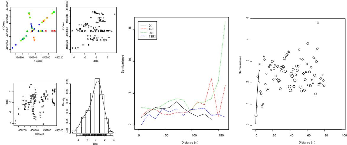
**Figure 8.** Left graphs: exploratory data analysis plots for residuals of temperature. Center graph: directional semivariograms for residuals of temperature. Right graph: empirical semivariogram (circles) and model (line) fit to residuals of temperature.
