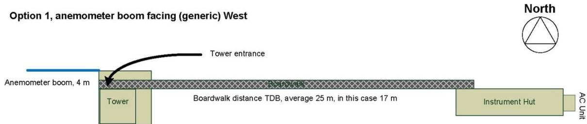
**Figure 57.** Generic diagram to demonstration the relationship between tower and instrument hut when boom facing west and instrument hut on the east towards the tower.
