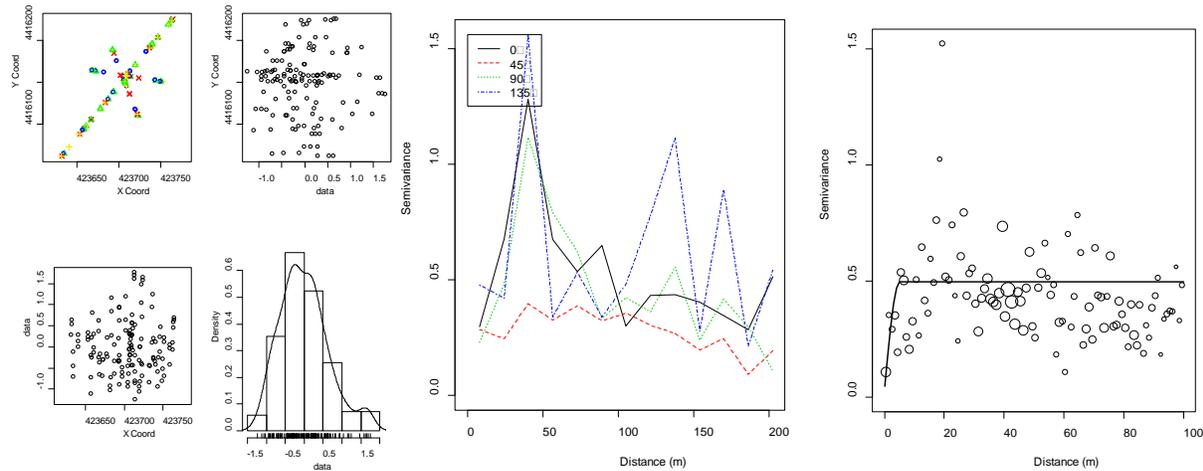
**Figure 48.** Left graphs: exploratory data analysis plots for residuals of temperature. Center graph: directional semivariograms for residuals of temperature. Right graph: empirical semivariogram (circles) and model (line) fit to residuals of temperature.
