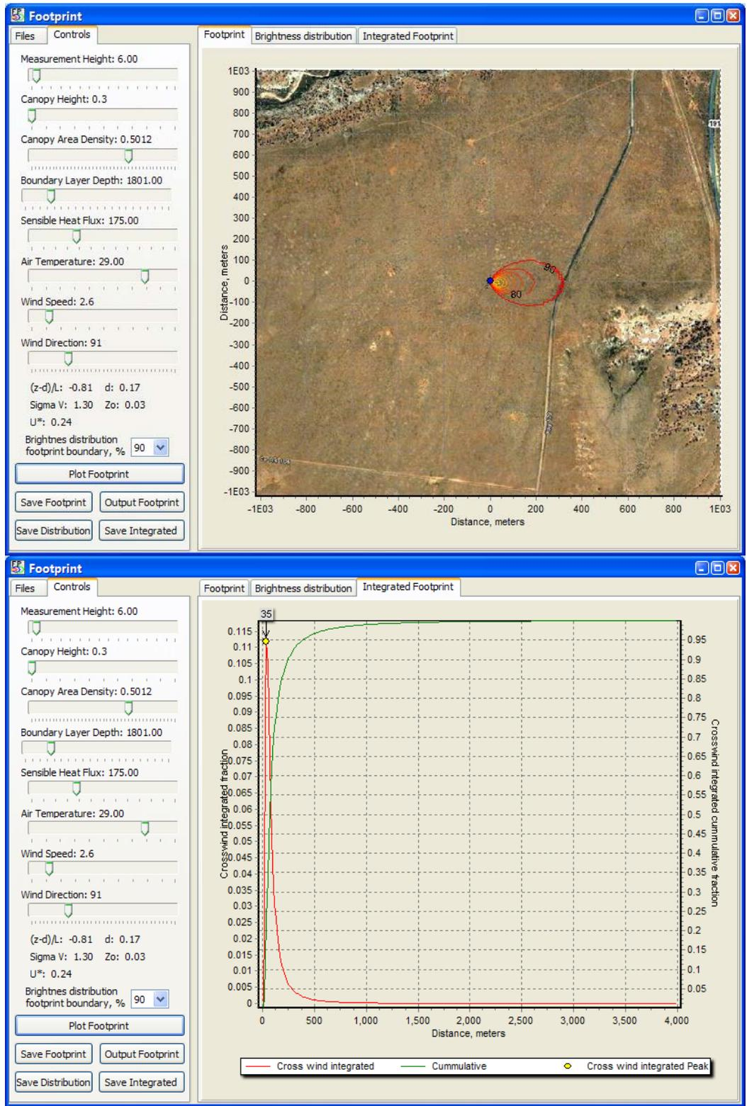
Figure 35. Moab Relocatable site summer nighttime (stable) footprint output with mean wind speed.
