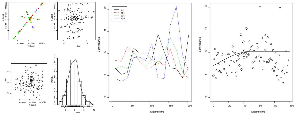
**Figure 50.** Left graphs: exploratory data analysis plots for residuals of soil water content. Center graph: directional semivariograms for residuals of water content. Right graph: empirical semivariogram (circles) and model (line) fit to residuals of water content.
