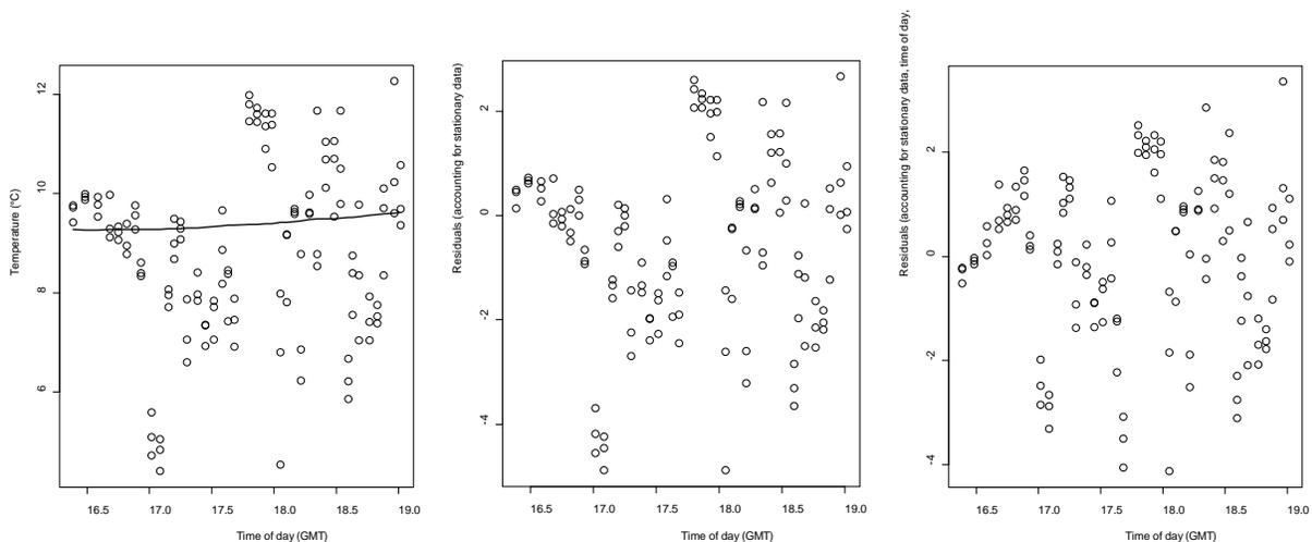
**Figure 7.** Left graph: mobile (circles) and stationary (line) soil temperature data. Center graph: temperature data after correcting for changes in temperature in the stationary data (circles) and a linear regression based on time of day (line). Right graph: residual temperature data after correcting for changes temperature in the stationary data and the time of day regression. Data in the right graph were used for the semivariogram analysis.
