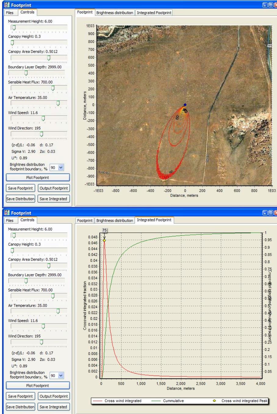
Figure 33. Moab Relocatable site summer daytime (convective) footprint output with max wind speed
