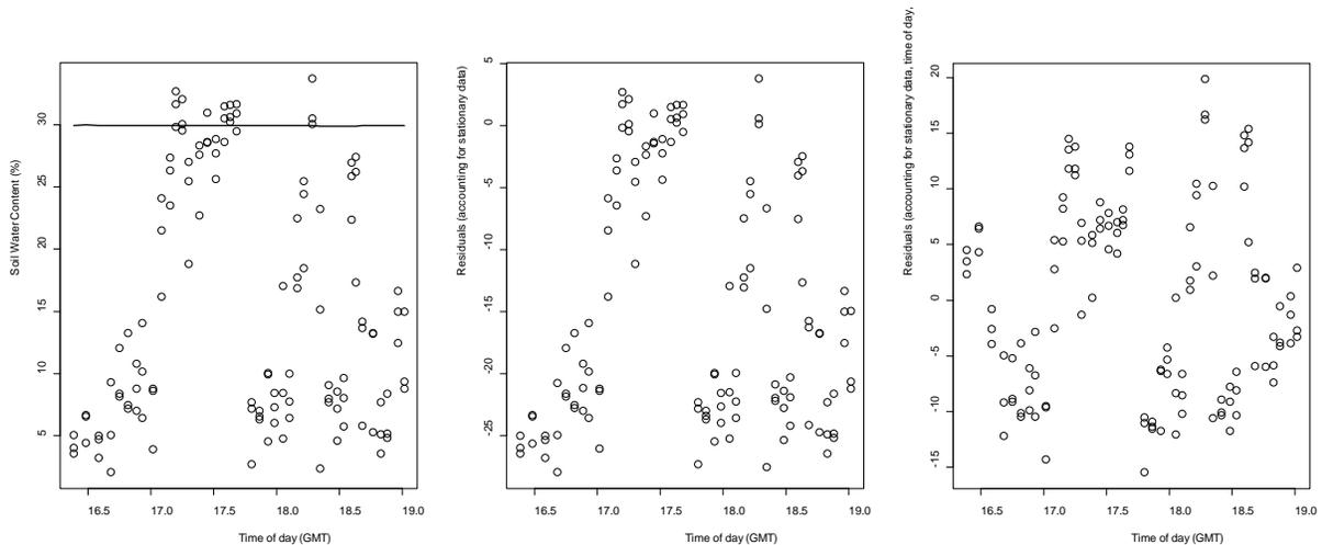
**Figure 9.** Left graph: mobile (circles) and stationary (line) soil water content data. Center graph: water content data after correcting for changes in water content in the stationary data (circles) and a linear regression based on time of day (line). Right graph: residual water content data after correcting for
