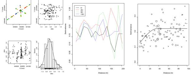
**Figure 30**. Left graphs: exploratory data analysis plots for residuals of soil water content. Center graph: directional semivariograms for residuals of water content. Right graph: empirical semivariogram (circles) and model (line) fit to residuals of water content.
