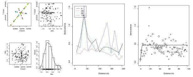
**Figure 48**. Left graphs: exploratory data analysis plots for residuals of temperature. Center graph: directional semivariograms for residuals of temperature. Right graph: empirical semivariogram (circles) and model (line) fit to residuals of temperature.
