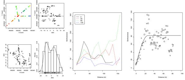
**Figure 10**. Left graphs: exploratory data analysis plots for residuals of soil water content. Center graph: directional semivariograms for residuals of water content. Right graph: empirical semivariogram (circles) and model (line) fit to residuals of water content.
