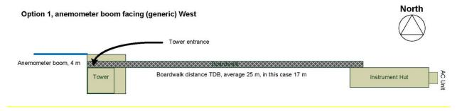
**Figure 57.** Generic diagram to demonstration the relationship between tower and instrument hut when boom facing west and instrument hut on the east towards the tower.
