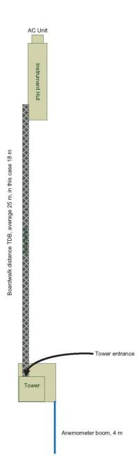
Figure 40. Generic diagram to demonstration the relationship between tower and instrument hut when boom facing south and instrument hut on the north towards the tower.
