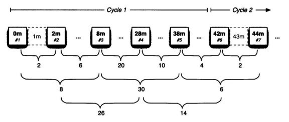
**Figure 46.** Spatially cyclic sampling design for the measurements of soil temperature and soil water content.
