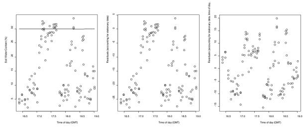
**Figure 9**. Left graph: mobile (circles) and stationary (line) soil water content data. Center graph: water content data after correcting for changes in water content in the stationary data (circles) and a linear regression based on time of day (line). Right graph: residual water content data after correcting for
