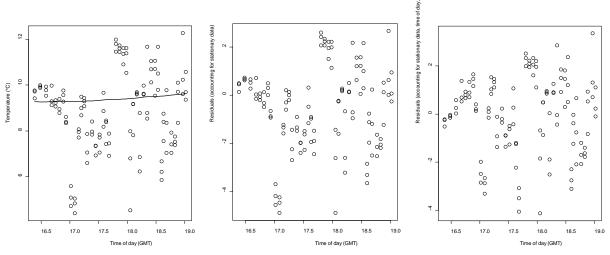
**Figure 7**. Left graph: mobile (circles) and stationary (line) soil temperature data. Center graph: temperature data after correcting for changes in temperature in the stationary data (circles) and a linear regression based on time of day (line). Right graph: residual temperature data after correcting for changes temperature in the stationary data and the time of day regression. Data in the right graph were used for the semivariogram analysis.
