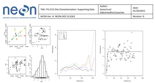
**Figure 8**. Left graphs: exploratory data analysis plots for residuals of temperature. Center graph: directional semivariograms for residuals of temperature. Right graph: empirical semivariogram (circles) and model (line) fit to residuals of temperature.
