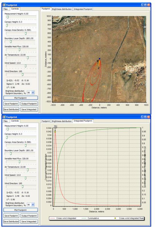
Figure 36. Moab Relocatable site winter daytime (convective) footprint output with max wind speed
