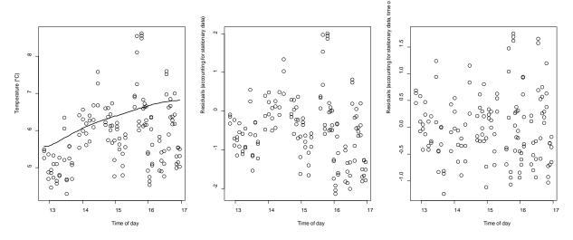
**Figure 47**. Left graph: mobile (circles) and stationary (line) soil temperature data. Center graph: temperature data after correcting for changes in temperature in the stationary data (circles) and a linear regression based on time of day (line). Right graph: residual temperature data after correcting for changes temperature in the stationary data and the time of day regression. Data in the right graph were used for the semivariogram analysis.
