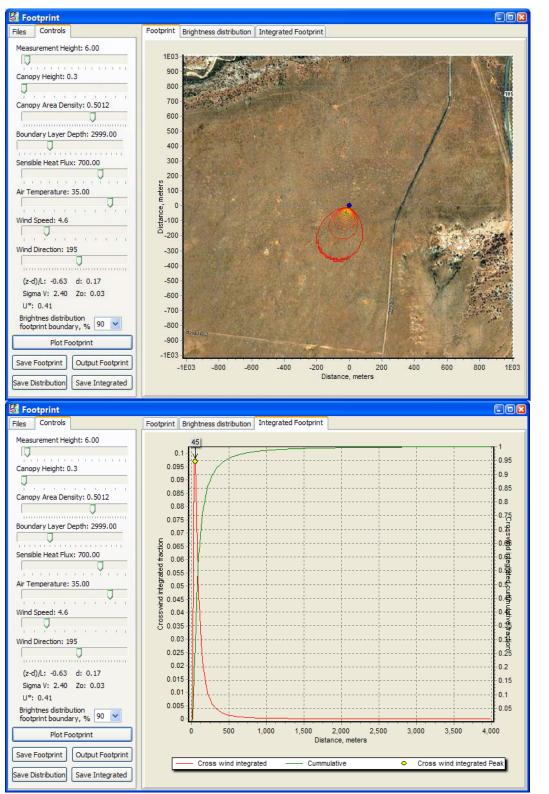
Figure 34. Moab Relocatable site summer daytime (convective) footprint output with mean wind speed
