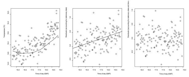
**Figure 27**. Left graph: mobile (circles) and stationary (line) soil temperature data. Center graph: temperature data after correcting for changes in temperature in the stationary data (circles) and a linear regression based on time of day (line). Right graph: residual temperature data after correcting for changes temperature in the stationary data and the time of day regression. Data in the right graph were used for the semivariogram analysis.
