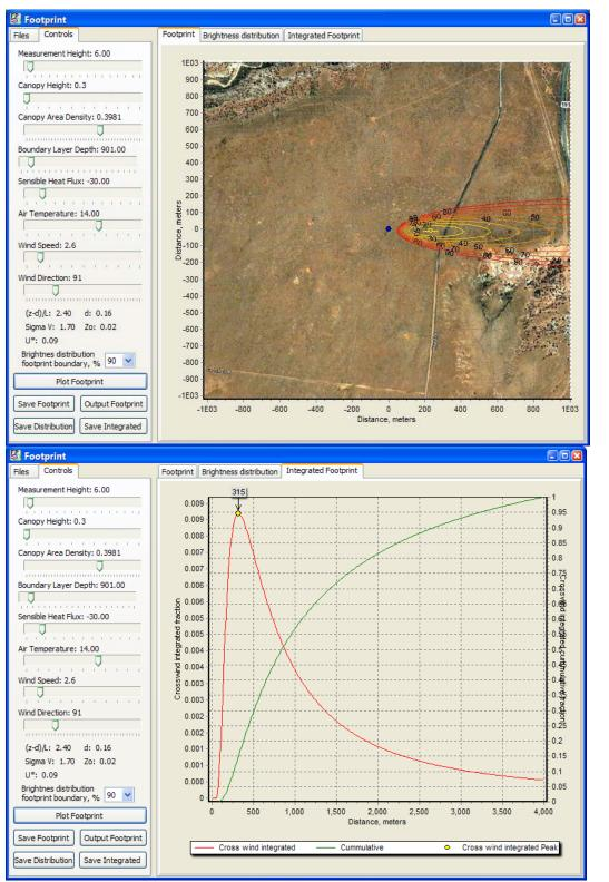
Figure 38. Moab Relocatable site winter nighttime (stable) footprint output with mean wind speed.
