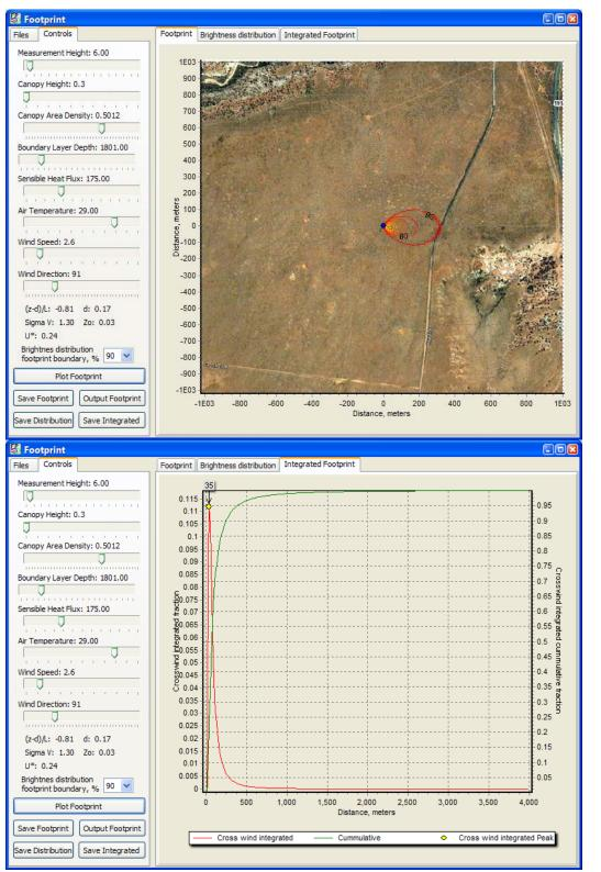
Figure 35. Moab Relocatable site summer nighttime (stable) footprint output with mean wind speed.
