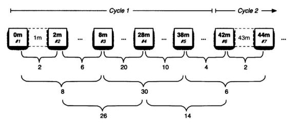
**Figure 6.** Spatially cyclic sampling design for the measurements of soil temperature and soil water content.
