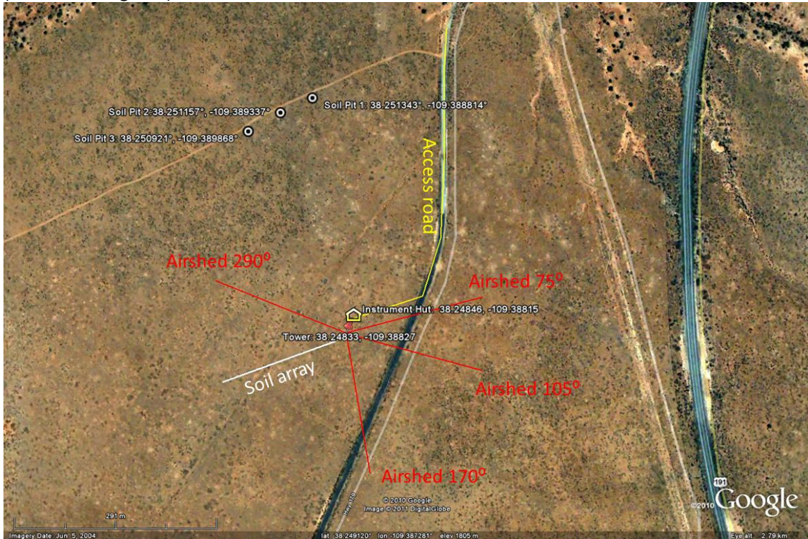
Figure 4. Site layout for Moab Relocatable site.
