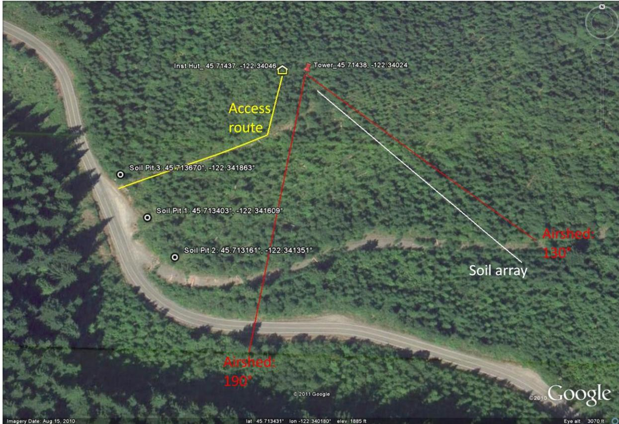
**Figure 45.** Site layout for Thayer Relocatable site.
