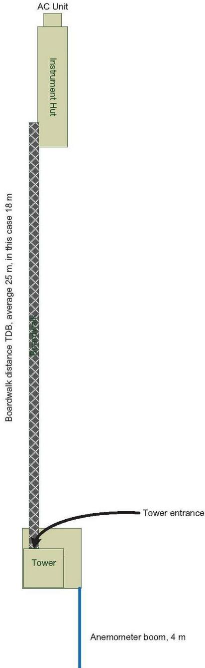
**Figure 72.** Generic diagram to demonstration the relationship between tower and instrument hut when boom facing south and instrument hut on the north towards the tower.
