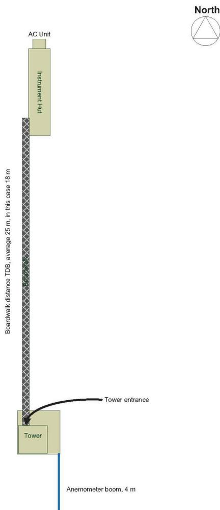
**Figure 46.** Generic diagram to demonstration the relationship between tower and instrument hut when boom facing south and instrument hut on the north towards the tower.
