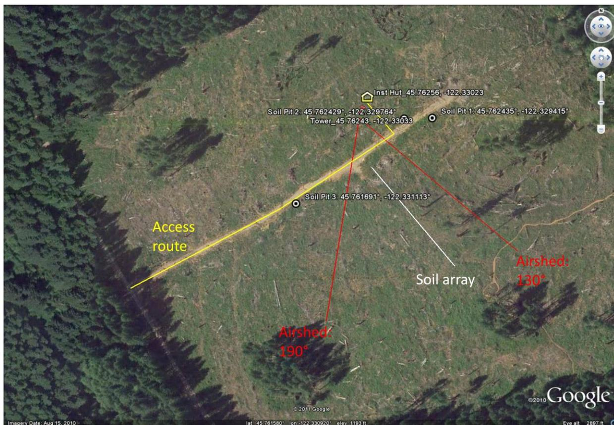
**Figure 57.** Site layout at Abby Road showing soil array and location of the FIU soil pit.
