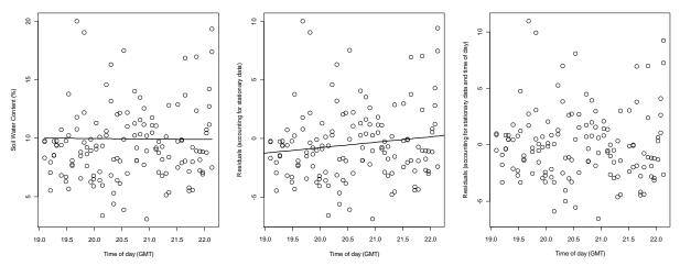
**Figure 9**. Left graph: mobile (circles) and stationary (line) soil water content data. Center graph: water content data after correcting for changes in water content in the stationary data (circles) and a linear regression based on time of day (line). Right graph: residual water content data after correcting for changes water content in the stationary data and the time of day regression. Data in the right graph were used for the semivariogram analysis.
