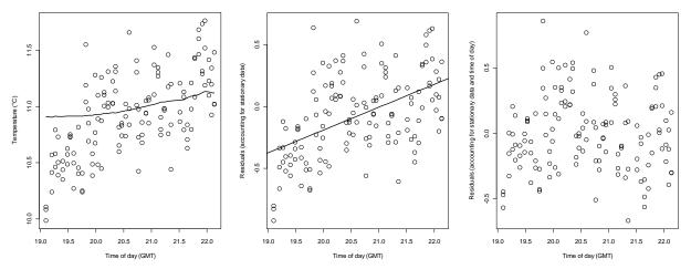
**Figure 7**. Left graph: mobile (circles) and stationary (line) soil temperature data. Center graph: temperature data after correcting for changes in temperature in the stationary data (circles) and a linear regression based on time of day (line). Right graph: residual temperature data after correcting for changes temperature in the stationary data and the time of day regression. Data in the right graph were used for the semivariogram analysis.
