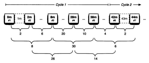
**Figure 26.** Spatially cyclic sampling design for the measurements of soil temperature and soil water content.
