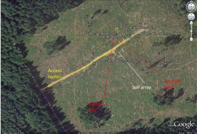
Figure 71. Site layout for Abby Road Relocatable site.
