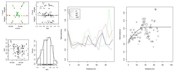
**Figure 28**. Left graphs: exploratory data analysis plots for residuals of temperature. Center graph: directional semivariograms for residuals of temperature. Right graph: empirical semivariogram (circles) and model (line) fit to residuals of temperature.
