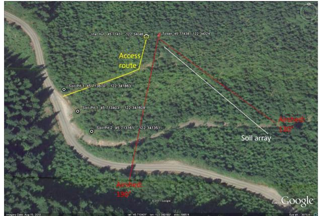
Figure 31. Site layout at Thayer showing soil array and location of the FIU soil pit.
