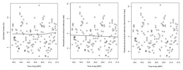
**Figure 55**. Left graph: mobile (circles) and stationary (line) soil water content data. Center graph: water content data after correcting for changes in water content in the stationary data (circles) and a linear regression based on time of day (line). Right graph: residual water content data after correcting for changes water content in the stationary data and the time of day regression. Data in the right graph were used for the semivariogram analysis.
