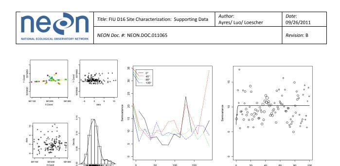
**Figure 10**. Left graphs: exploratory data analysis plots for residuals of soil water content. Center graph: directional semivariograms for residuals of water content. Right graph: empirical semivariogram (circles) and model (line) fit to residuals of water content.
