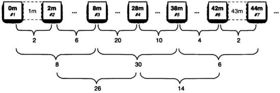
**Figure 6.** Spatially cyclic sampling design for the measurements of soil temperature and soil water content.
