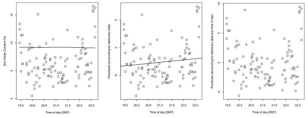
**Figure 29**. Left graph: mobile (circles) and stationary (line) soil water content data. Center graph: water content data after correcting for changes in water content in the stationary data (circles) and a linear regression based on time of day (line). Right graph: residual water content data after correcting for changes water content in the stationary data and the time of day regression. Data in the right graph were used for the semivariogram analysis.
