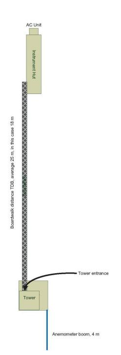
**Figure 72.** Generic diagram to demonstration the relationship between tower and instrument hut when boom facing south and instrument hut on the north towards the tower.
