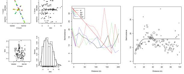
**Figure 56**. Left graphs: exploratory data analysis plots for residuals of soil water content. Center graph: directional semivariograms for residuals of water content. Right graph: empirical semivariogram (circles) and model (line) fit to residuals of water content.
