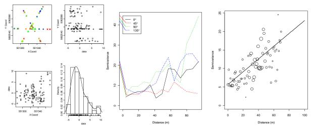
**Figure 30**. Left graphs: exploratory data analysis plots for residuals of soil water content. Center graph: directional semivariograms for residuals of water content. Right graph: empirical semivariogram (circles) and model (line) fit to residuals of water content.
