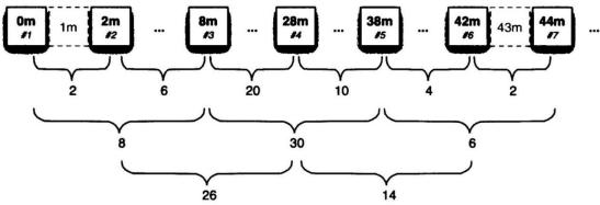
**Figure 52.** Spatially cyclic sampling design for the measurements of soil temperature and soil water content.
