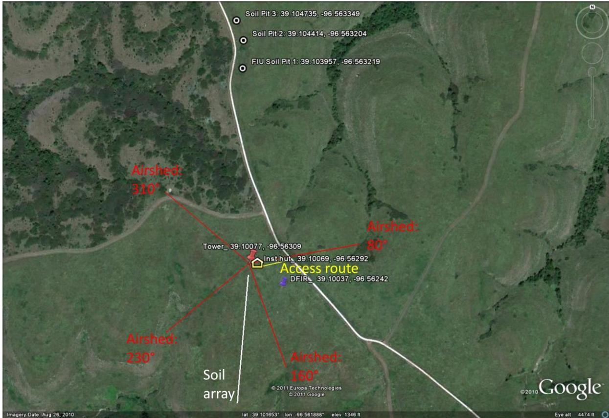
**Figure 11.** Site layout at Konza - Core showing soil array and location of the FIU soil pit.
