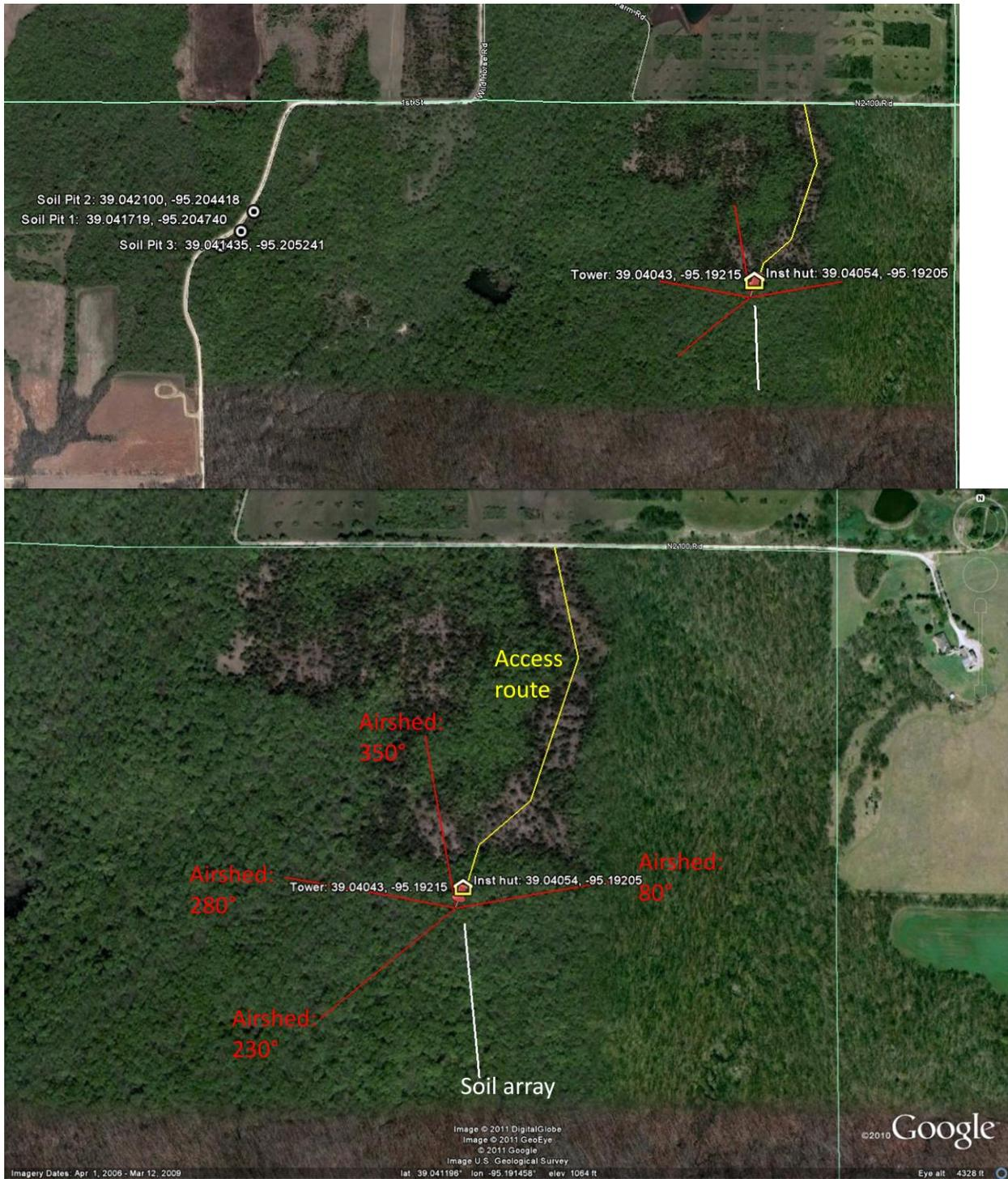
**Figure 31.** Site layout at University of Kansas Biological Station showing soil array and location of the FIU soil pit. Soil pits are ~1 km from tower as this was the closest location to the tower with good road access for a bobcat-type excavator with the same soil type
