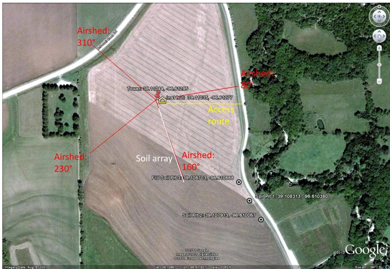
**Figure 51.** Site layout at Konza - Relocatable showing soil array and location of the FIU soil pit.
