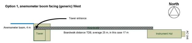
**Figure 20.** Generic diagram to demonstration the relationship between tower and instrument hut when boom facing west and instrument hut on the east towards the tower.
