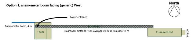
**Figure 60.** Generic diagram to demonstration the relationship between tower and instrument hut when boom facing west and instrument hut on the east towards the tower.
