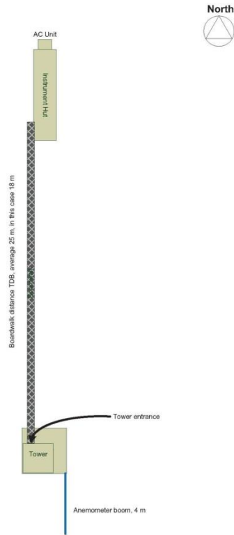
Figure 1. Generic diagram to demonstrate the relationship between tower and instrument hut when boom is facing south and instrument hut is on the north towards the tower. This is just a generic diagram. The actual layout of boardwalk (or path if no boardwalk required) and instrument hut position will be the joint responsibility of FCC and FIU. At this site, the boom angle will be 205 degrees. The instrument hut location is on the northwest toward tower; the distance between instrument hut and tower is 20 m. The instrument hut vector will be E-W (90°-270°, longwise).
