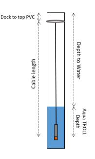
Cable length + Dock to top PVC = Depth to water + Aqua Troll Depth
