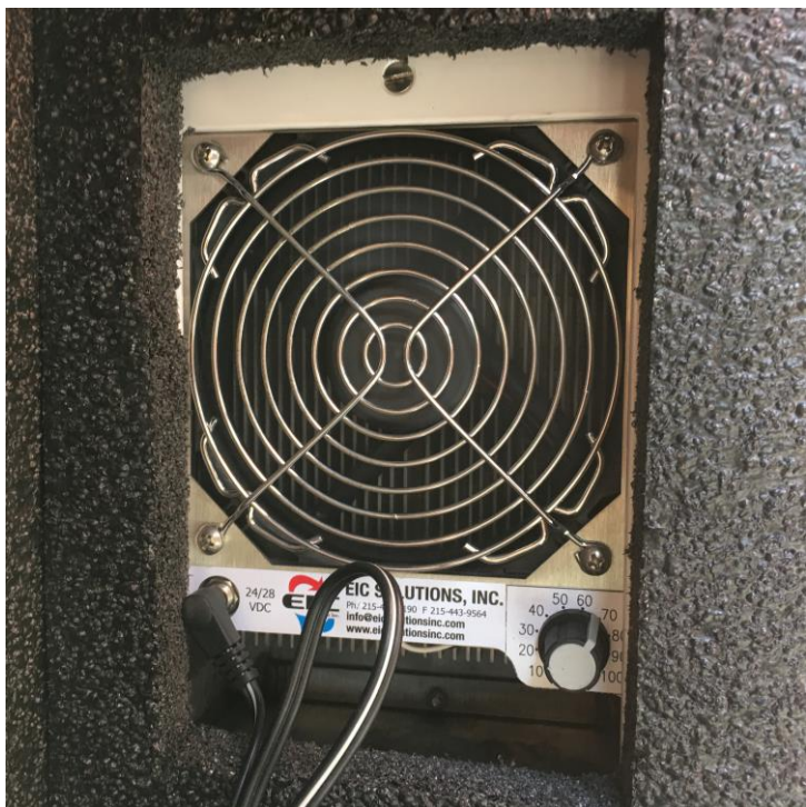
Figure 9. View of the Thermo-electric chiller unit from inside the enclosure (see Figure 5j for its location).
