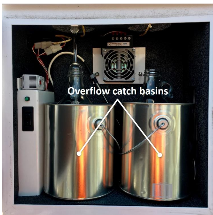
Figure 6. Overflow catch basins placement.
