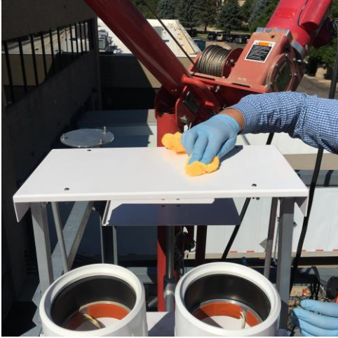
Step 6. Clean the top surface of the Moving Cover.
