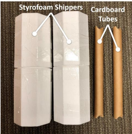
Figure 19. Internal packaging for the glassware shipping boxes.
