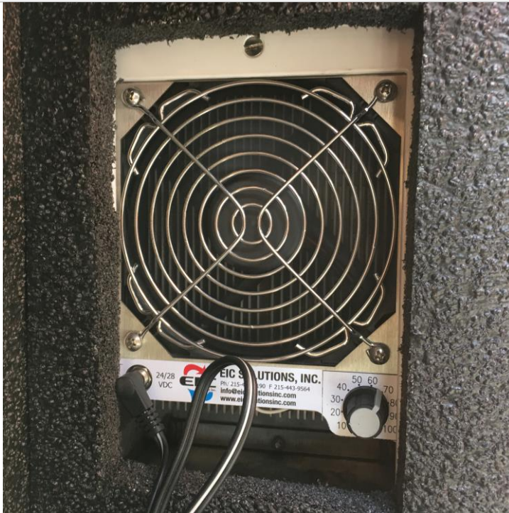
Figure 10. View of the Thermo-electric chiller unit from inside the enclosure (see Figure 5 for its location).
