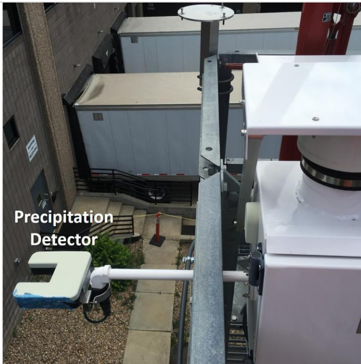
Figure 4. A view of the precipitation detector. This unit is typically located on an extension arm projecting from the environmental enclosure.
