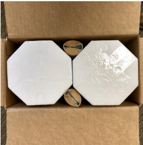
Figure 25. Placement of the Styrofoam shippers and the cardboard tubes within the glassware shipping box.
