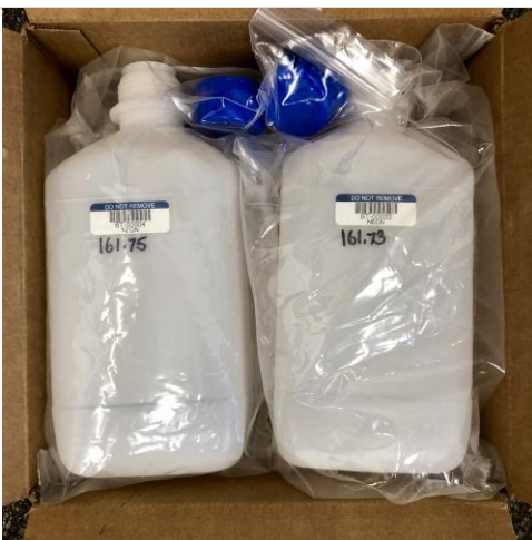
Figure 26. The plastic shipping bottles are packed within plastic reclosable bags and side-by-side within their own shipping box.
