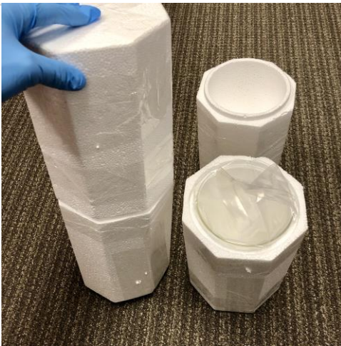
Figure 22. The half without the ridges will go over the funnel side and then packed into the shipping box (see Figure 25 ).
