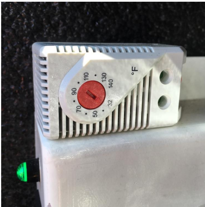
Figure 9. A view of one of the internal Temperature Controllers. See Figure 5 for the location of this Temperature Controller.
