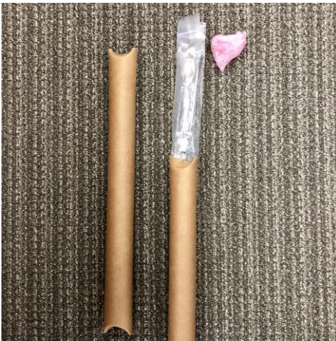
Figure 24. The thistle tubes are placed inside a plastic bag and then within the cardboard tube.
