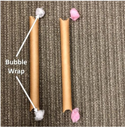
Figure 23. The cardboard tubes will have bubble wrap or foam bits at each end to minimize the movement of the thistle tube within the cardboard tube.
