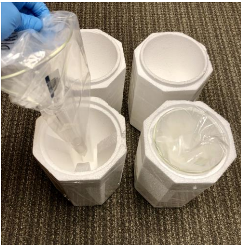
Figure 21. The narrow end of the funnels will go inside the half with the ridges.
