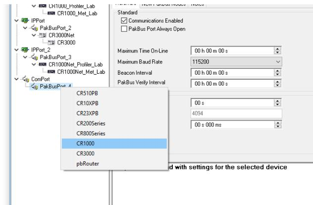
l) With CR1000 selected, click Rename in the main toolbar and change the name to CR1000\_Profiler and in the Hardware tab, change the “PakBus Address” to 10
