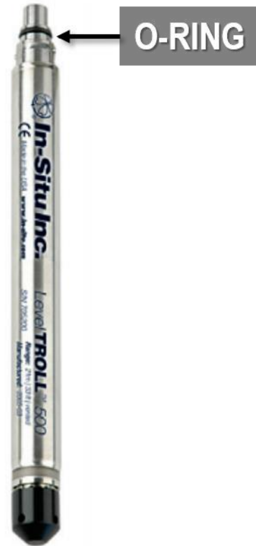
Figure 8. O-Ring Location on Level TROLL Sensor
