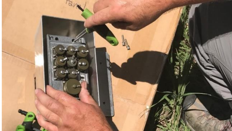
Figure 10. Remove Grape from Grape Shields (D06 KING)
