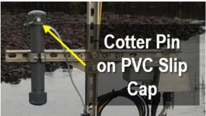
Figure 19. A Slip Cap with Cotter Pin Secures Desiccant PVC Housing
