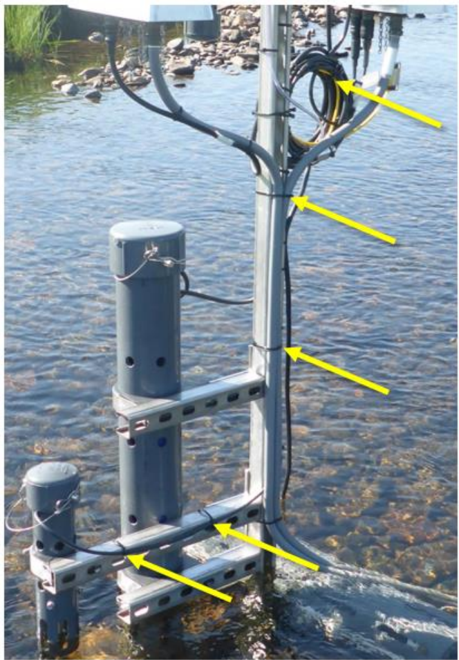
Figure 23. Secure Cables using Zip Ties (D18 OKSR)
