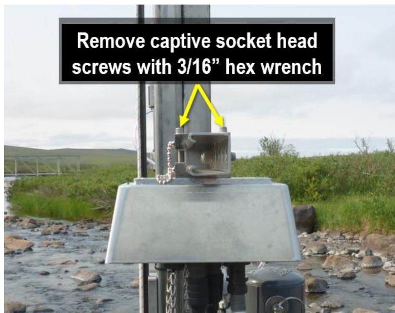
Figure 11. Remove Grape Shield with 3/16" Hex Wrench
