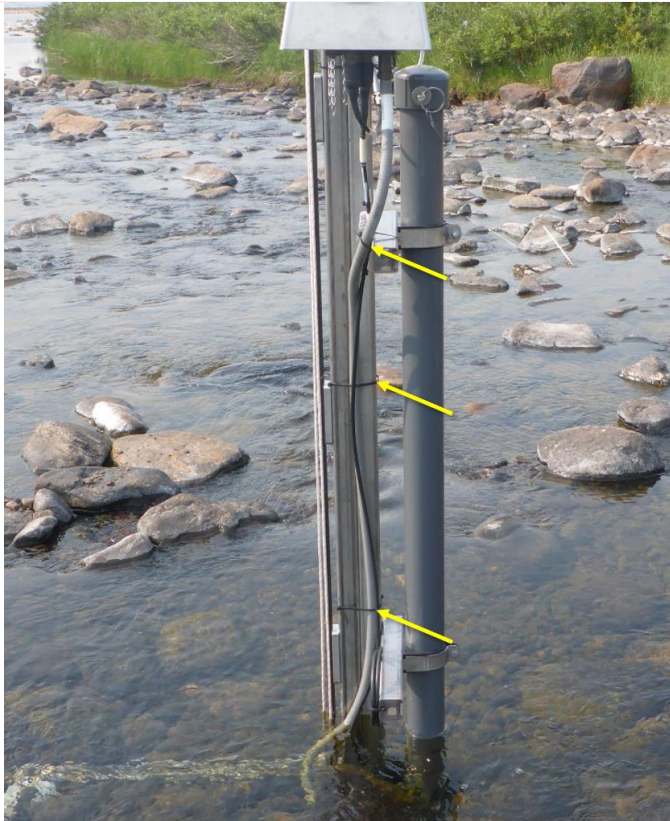
Figure 18. Secure Cables using Zip Ties
