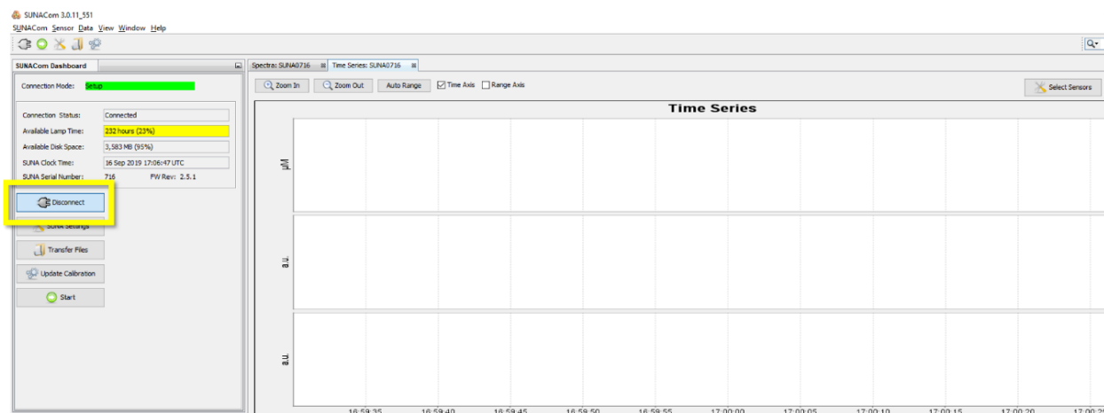
Figure 8. Disconnect the SUNA from the UCI Software FIRST, and then Disconnect the SUNA Physically
