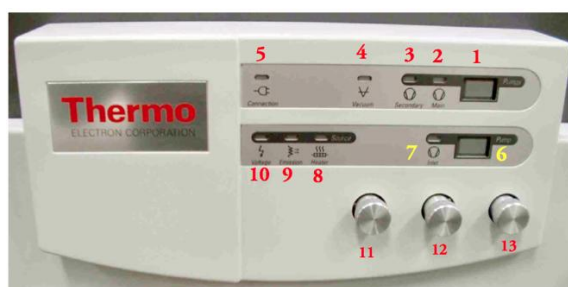
Figure 11. Delta V control panel (from the Thermo user manual).
