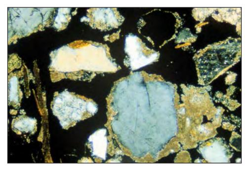
Figure 3E1-7.—Calcium carbonate around quartz and feldspar grains in a chitonic c/f related distribution pattern. The calcite has characteristic high birefringence under cross-polarized light. This is the Bkq2 horizon in a Cax soil (pedon 97P0420) from San Bernardino, CA. Frame width is 0.9 mm.
