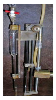
Figure 3A-2.—Close-up of the Shaw Pipette apparatus.
