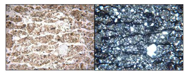
Figure 3E1-12.—Voids termed "planes" that developed in the platy structure of the A1 horizon in a Frisite soil (pedon 98P0453) from Wyoming. The image on the left is under plane-polarized light, and the image on the right is under cross-polarized light. Frame width is 2.5 mm.
