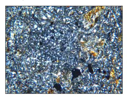
Figure 3E1-16.—A stipple speckled b-fabric under cross-polarized light from the BE horizon in an Adco soil (pedon 87P0771), which is a Vertic Albaqualf, from Macon County, Missouri. The horizon consists of 29% clay and 63% silt. It has a COLE of 0.026 and a clay fraction dominated by smectite with lesser amounts of mica and kaolinite. Frame width is 1.3 mm.
