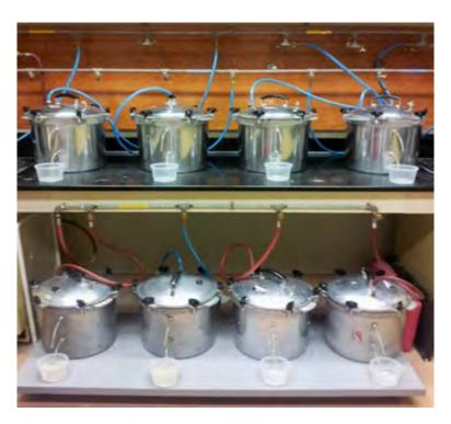
Figure 3C1a-2.—Pressure-plate extraction at 33 kPa for clods.
