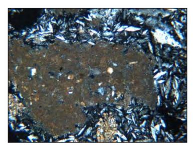
Figure 3E1-8.—Lenticular gypsum crystals surrounding a micritic calcite mass under cross-polarized light. This is the Bym1 horizon in a Drygyp soil (pedon 04N0770) from Nevada. Frame width is 2.5 mm.
