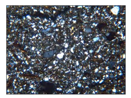
Figure 3E1-15.—A speckled b-fabric under cross-polarized light in an Ap horizon of a Typic Argiudoll. The soil is in the Southridge series (pedon 87P0075) from Allamakee County, lowa. This horizon has 19% clay and a COLE of 0.016. The clay fraction is dominated by vermiculate and smectite. Frame width is 1.3 mm.
