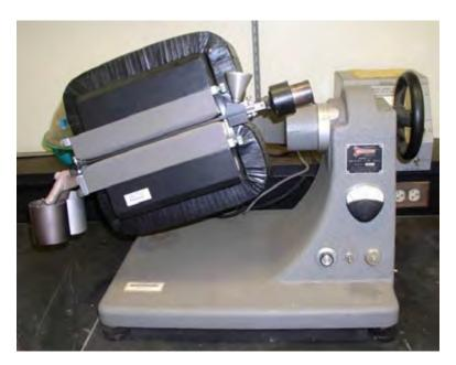
Figure 7B2-1.—Apparatus for magnetic separation.
