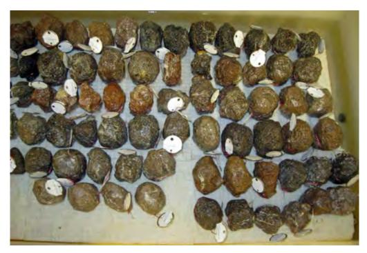
Figure 3B1b-2.—After a flat surface on the clod is cut with a diamond saw, the clod is placed on a tension table, maintained at 5-cm tension.
