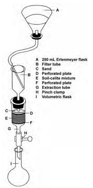
Figure 6N3-1.—Apparatus for ammonium chloride-ethanol extraction for calcium (6N3).
