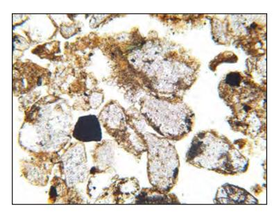
Figure 3E1-9.—Simple packing voids, partially coated with fine materials under plane-polarized light. These voids arise from loose packing of soil components. This is the Bt1 horizon in an Endlich soil (pedon 99P0001) from Colorado. Frame width is 1.1 mm.
