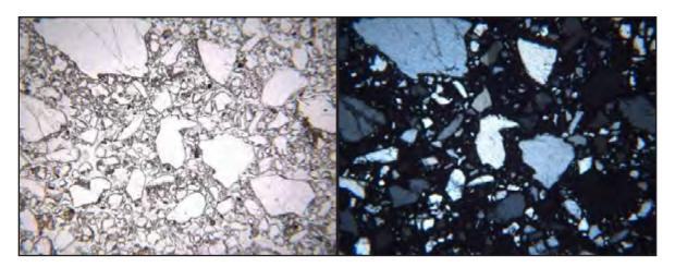
Figure 3E1-14.—An example of the enaulic c/f related distribution pattern under plane-polarized light (left) and cross-polarized light (right). The image is of an E horizon in a Fuquay soil (pedon 06N0830) from South Carolina. The soil is a Kandiudult. Frame width is 2.5 mm.
