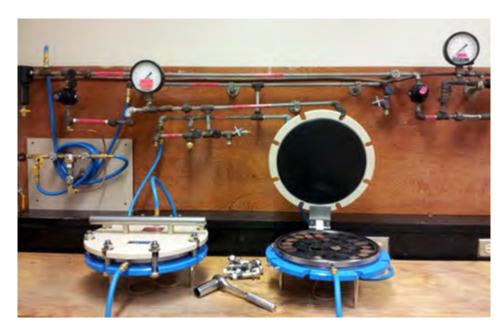
Figure 3C2a-1.—Sieved (<2-mm) soil placed in pressure-membrane extractor.
