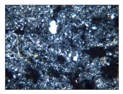
Figure 3E1-17.—A mosaic speckled b-fabric under crosspolarized light of the 2Btg3 horizon in a Leonard soil (Pedon 87P0770), which is a Chromic Vertic Epiaqualf, from Macon County, Missouri. Frame width is 1.1 mm. This horizon has 48% clay, a COLE of 0.132, and a clay fraction dominated by smectite.
