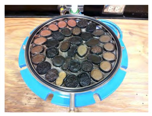
Figure 3C2a-2.—Pressure-membrane extraction at 1500-kPa for <2-mm samples.
