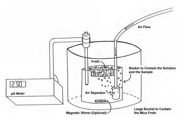
Figure 7B2c-1.—Apparatus for froth flotation.
