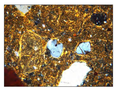
Figure 3E1-19.—A granostriated b-fabric under cross-polarized light of the Bt horizon in a Redding soil (Pedon 40A2847), which is a Durixeralf, from San Diego County, California. Frame width is 1.1 mm. This horizon has 60% clay, a COLE of 0.063, and a clay fraction dominated by kaolinite and smectite.
