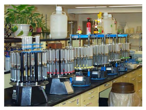
Figure 4B-2.—Mechanical vacuum extractors used at the USDA-NRCS Kellogg Soil Survey Laboratory for chemical extractions and analyses, e.g., cation exchange capacity, NH<sub>4</sub>OAc, pH 7.
