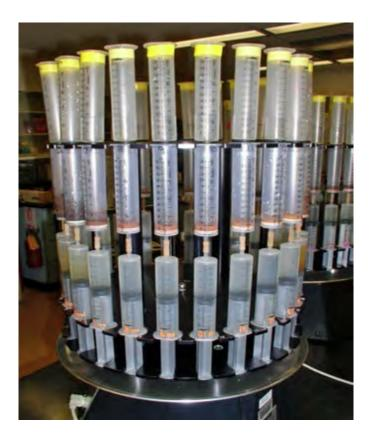
Figure 4B-1.—Mechanical vacuum extractor, Sampletek, Mavco Industries, Lincoln, NE.
