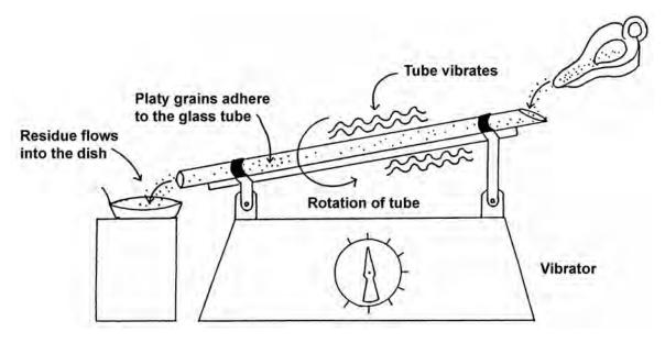
Figure 7B2b-1.—Apparatus for Static Tube Separation.
