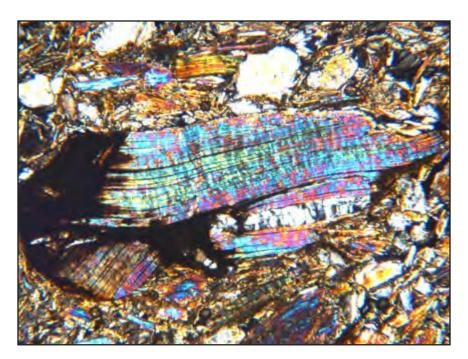
Figure 3E1-2.—Large biotite grain undergoing expansion from weathering. Note the high birefringence due to the orientation of the grain in thin section. Frame width is 1.1 mm. (Series name not designated; Fremont Co., WY; pedon 98P0456; Bt2 horizon under cross-polarized light).
