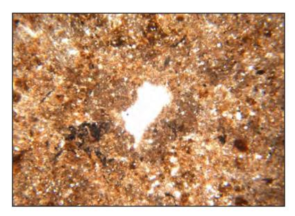
Figure 3E1-10.—A void (under plane-polarized light) that would be described as a vugh. Vughs are semi-equidimensional, irregular voids that are not interconnected with other voids. This photomicrograph is of the Bkss horizon of a Typic Epiaquert from Brazoria County, Texas (pedon 98P0582). This horizon is 52% clay and 42% silt. The COLE is 0.011, and the clay fraction is principally composed of smectite. Frame width is 2.5 mm.
