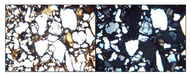
Figure 3E1-3.—A Btvx2 horizon in a pedon of Dothan soil (06N0831) in plane-polarized (left) and cross-polarized (right) light. The horizon has close porphyric c/f related distribution and a micromass that is composed of kaolinite embedded with Fe oxides. Note the yellow vermiform kaolinite in the right center of the image. This grain likely forms via in situ weathering of a sand-sized grain. Frame width is 2.5 mm.
