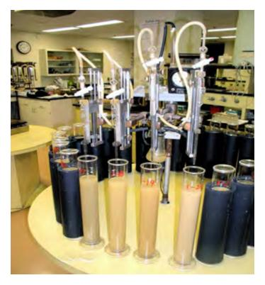
Figure 3A-3.—Shaw Pipette used for particle-size analysis of the <2-mm fraction at the USDA-NRCS Kellogg Soil Survey Laboratory.
