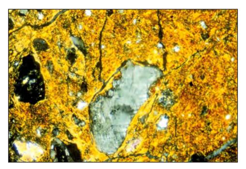
Figure 3E1-5.—A Btk2 horizon in a pedon of a White House soil (pedon 40A3559) under cross-polarized light. The horizon has a high percentage of clay of expandable aluminosilicate clay-sized minerals. Clays become aligned through shrink-swell processes. This alignment results in preferred orientation of clay particles, making the clay birefringent (visible under cross-polarized light). Shrinking and swelling results in a loss of clay coatings along ped faces in many soils. Frame width is 0.9 mm.
