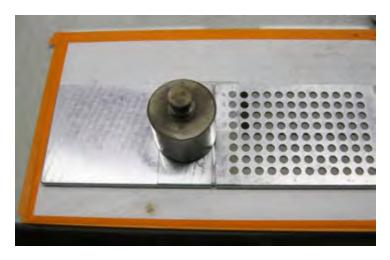
Figure 7A7-1.—Filled sample plate with glass plate covering leftmost two columns and with weight holding glass plate in place.
