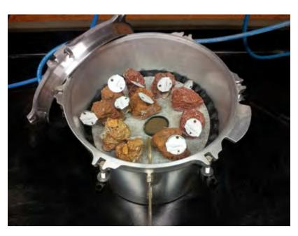
Figure 3C1a-1.—Clods in pressure-plate extractor following saturation.
