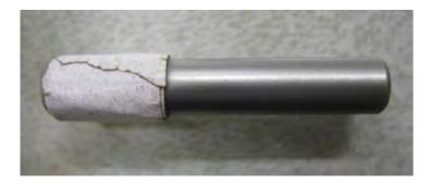
Figure 7A7-2.—Steel rod for packing sample plates.
