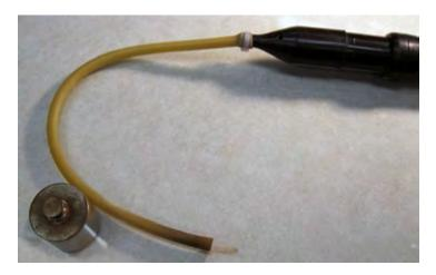
Figure 7A7-3.—Vacuum cleaner to clean sample plates.
