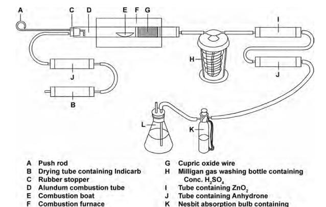
Figure 6A2b-1.—Apparatus used for organic carbon determination by dry combustion, carbon dioxide evolution II (6A2b).
