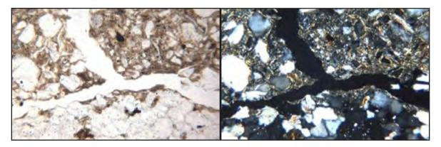
Figure 3E1-6.—The Bt1 horizon in a Brod soil (pedon 03N1014), a Ustollic Haplocryalf from Montana. Note the oriented clay around coarse grains (granostriated b-fabric) under plane-polarized light (left) and cross-polarized light (right). Frame width is 1.1 mm.
