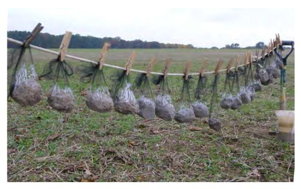
Figure 3B1a-2.—After dipping, clods are tied to clothesline to dry.
