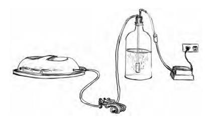
Figure 4C-1.—Apparatus for measuring oxidized pH.
