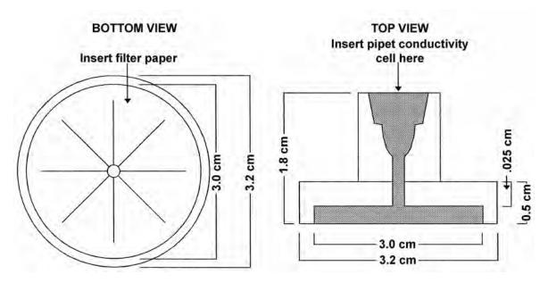
Figure 8a1b-1.—Miniature Richards-type extractor made of polymethyl methacrylate (Lucite).
