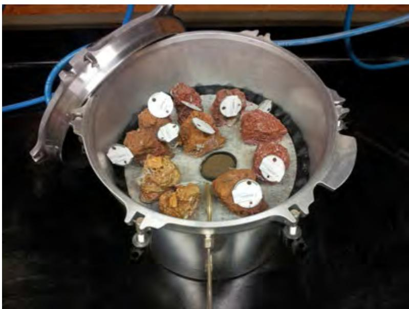
**Figure 3C1a-1.—Clods in pressure-plate extractor following saturation.**
