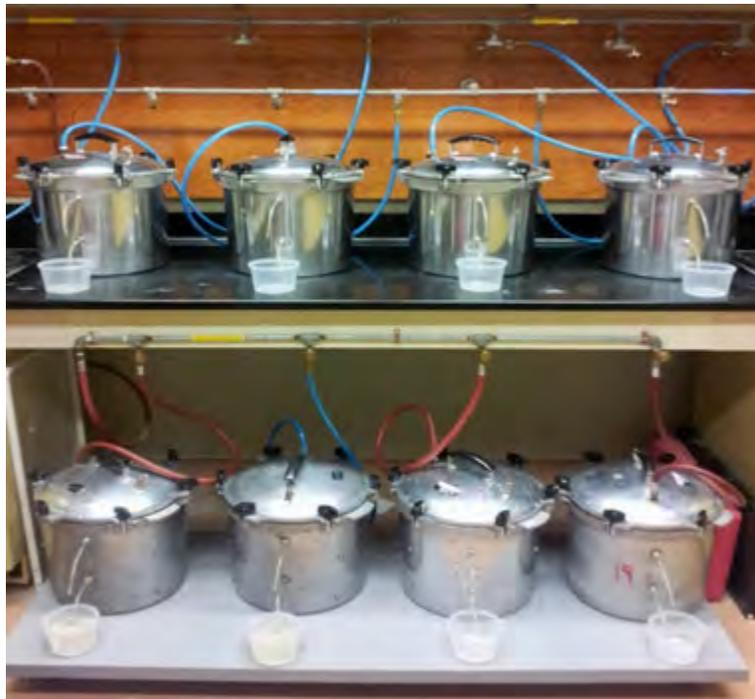
Figure 3C1a-2.—Pressure-plate extraction at 33 kPa for clods.
