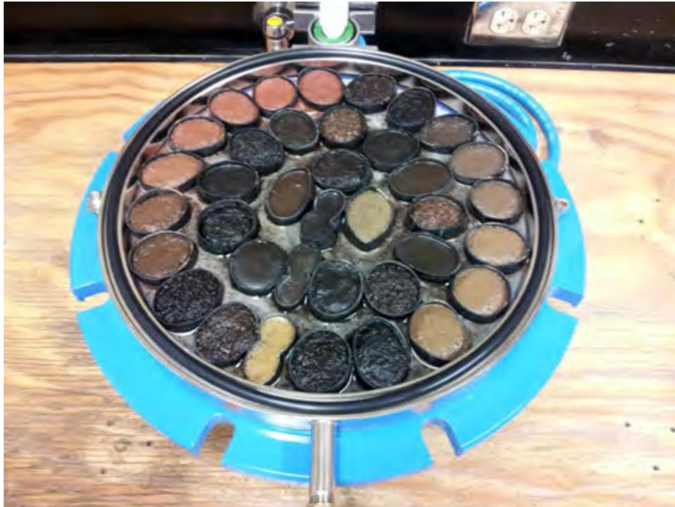
**Figure 3C2a-2.—Pressure-membrane extraction at 1500-kPa for <2-mm samples.**
