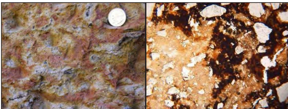
**Figure 3E1-21.—**The mottled fabric on the pit face (left) of a Btvx2 horizon in a Fuquay pedon, and the thin section of soil fabric (right) from the same horizon. These photos illustrate the movement of Fe oxides in the soil as it undergoes seasonal saturation and reduction followed by reoxidation.
