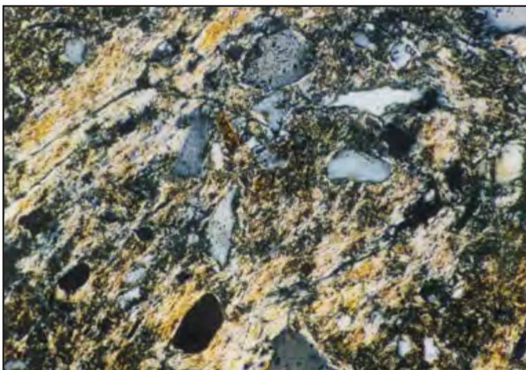
**Figure 3E1-18.—A parallel striated b-fabric under cross-polarized light of the Bt horizon in a Gloria soil (pedon 40A2845), which is a Durixeralf, from Monterey County, California. Frame width is 1.3 mm. This horizon has 47% clay, a COLE of 0.056, and has a clay fraction dominated by illite with lesser amounts of kaolinite and smectite.**
