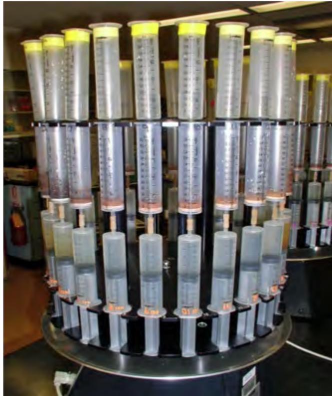
Figure 4B-1.—Mechanical vacuum extractor, Sampletek, Mavco Industries, Lincoln, NE.
