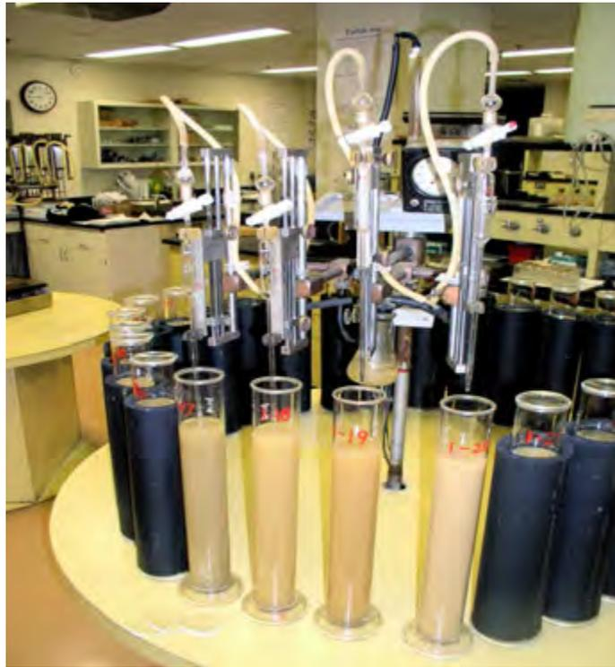
**Figure 3A-3.—Shaw Pipette used for particle-size analysis of the <2-mm fraction at the USDA–NRCS Kellogg Soil Survey Laboratory.**
