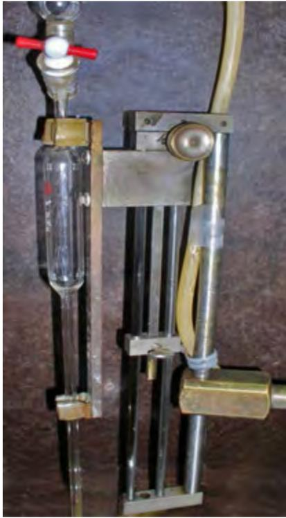
**Figure 3A-2.—Close-up of the Shaw Pipette apparatus.**
