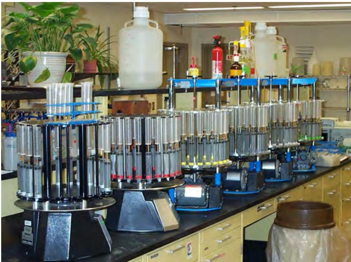
**Figure 4B-2.—Mechanical vacuum extractors used at the USDA–NRCS Kellogg Soil Survey Laboratory for chemical extractions and analyses, e.g., cation exchange capacity,  $\text{NH}_4\text{OAc}$ , pH 7.**
