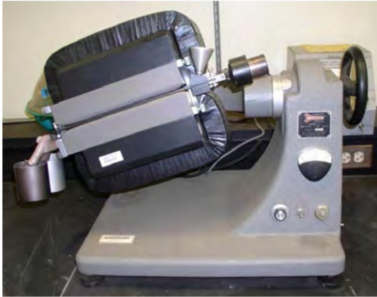
Figure 7B2-1.—Apparatus for magnetic separation.
