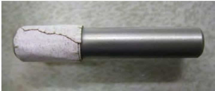
**Figure 7A7-2.—Steel rod for packing sample plates.**
