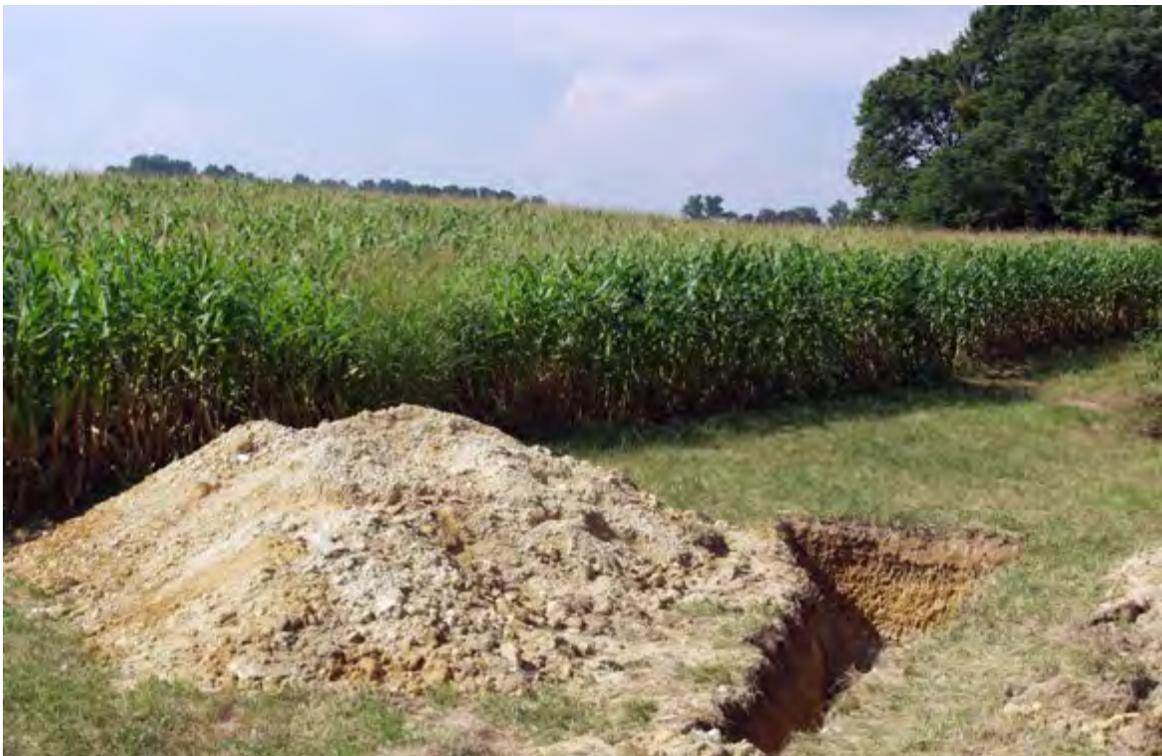
**Figure 1A-2.—Excavated pit for pedon sampling.**
