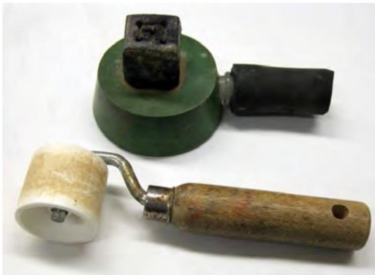
Figure 7A1-1.—Vacuum chuck (top) and slide roller (bottom).
