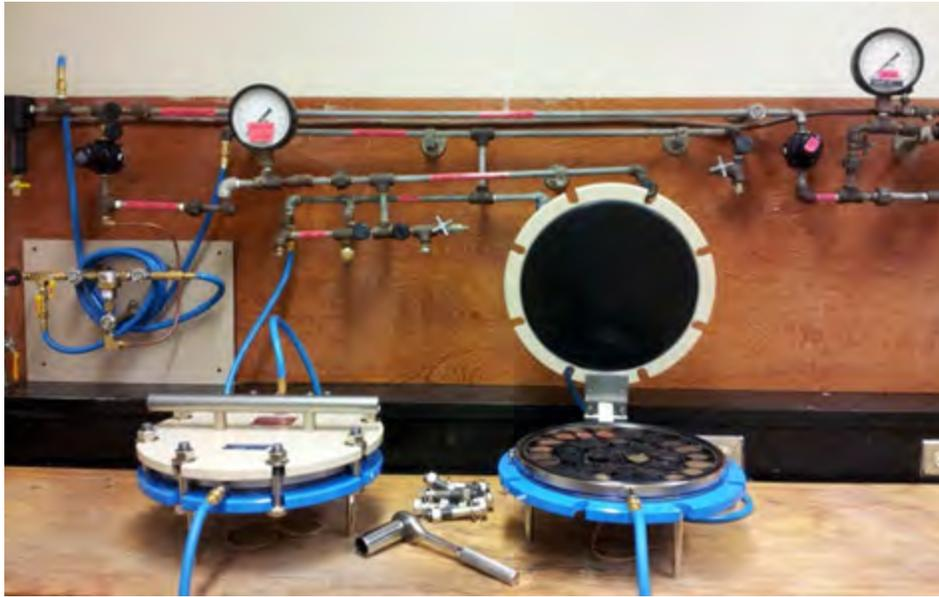
**Figure 3C2a-1.—Sieved (<2-mm) soil placed in pressure-membrane extractor.**
