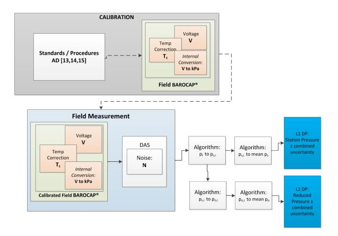
**Figure 1:** Displays the sources of uncertainty and data flow for L1 Station and reduced pressure DPs. The salmon colored boxes represent the measurement of pressure based on the theory of aneroid barometry. For more information regarding the calibration procedure, please refer to AD [13,14,15].
