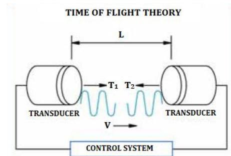
**Figure 1.** Ultrasonic anemometer theory (directionless) (Gill 2007).
