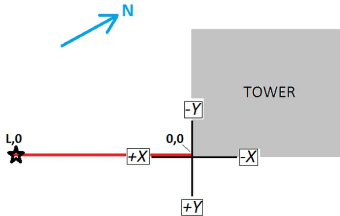
**Figure 4.** An example of the Cartesian coordinate system as used to calculate site-specific, distorted wind flow regions. The tower is shown as a gray square; the coordinate system is represented by the black lines; the 2D anemometer boom is given as a red line and the 2D anemometer is displayed as a black star. True North is denoted at the top of the Figure.
