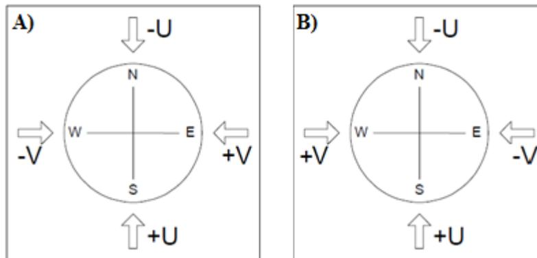
**Figure 2.** A) Coordinate system of an upright sonic anemometer (Gill 2007, 2011) used at Aquatic Sites; B) coordinate system of Gill’s 2D sonic anemometer oriented upside-down used at Terrestrial Sites - it is important to note that the zonal plane is flipped because one of the transducer arms must be aligned with True North during installation.
