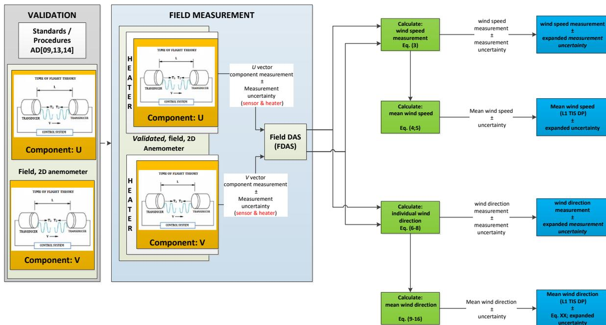
**Figure 5.** Diagram outlining potential sources of uncertainty associated with 2D wind L1 DPs. The salmon colored boxes represent the direct measurement of vector velocity based on the theory of sonic anemometry. For more information regarding the validation procedure, please refer to AD[09,13,14]
