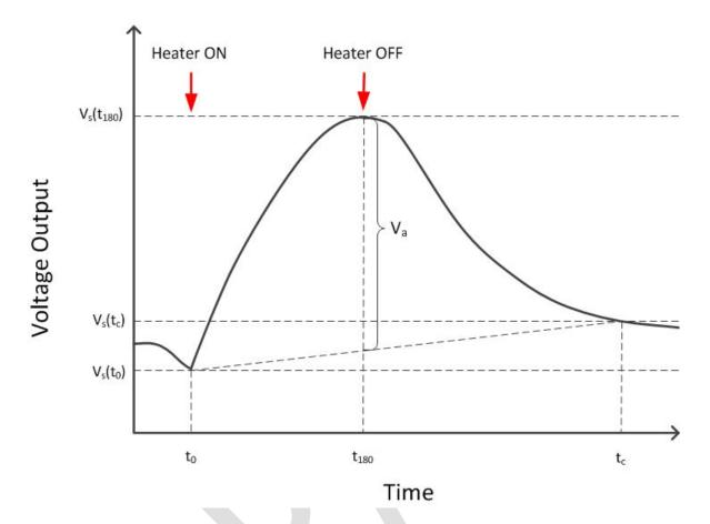
Figure 2. A conceptual plot of the voltage output ( $V_s$ ) from the sensor when performing a self-calibration. After the sensor response to self-heating ( $V_a$ ) is obtained, the *in-situ* correction factor ( $E_f$ ; V/Wm<sup>-2</sup>) for the plate is then estimated as:
