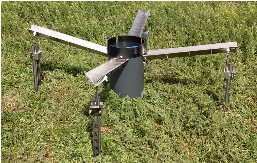
Figure 2: Image of a modified Met One tipping bucket sensor to collect throughfall in the field.
