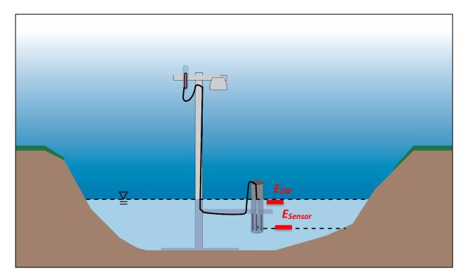
**Figure 5.** Illustration showing the location of the Elevation of the sensor ( $E_{Sensor}$ ) which is measured by SI&V and the calculated Surface Water Elevation ( $E_{SW}$ ).
