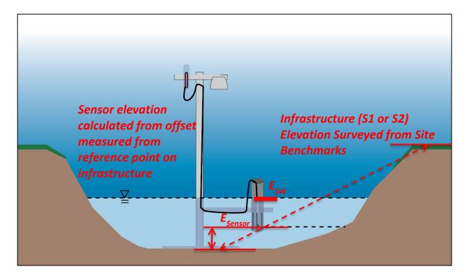
Figure 7. Illustration of the points measured by SI&V during installation in order to calculate the sensor elevation.
