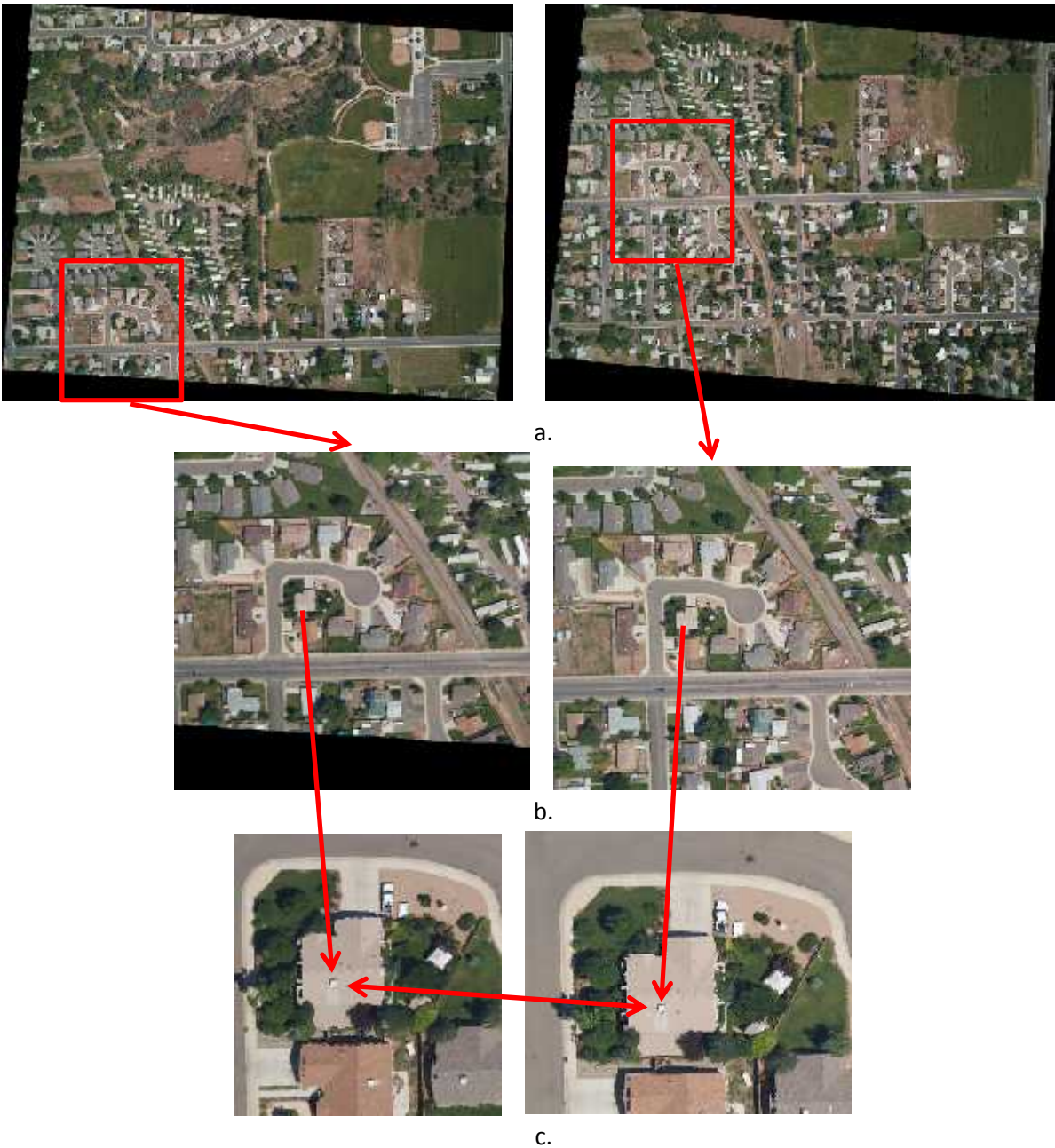
Figure 8. Two overlapping digital images showing a tie point: full images, b. zoom level 1, c. zoom level 2. The red boxes enclose the same areas in each image. The red arrows connect the tie point, a white object on top of a roof.
