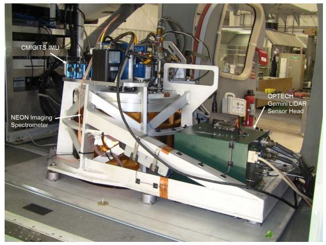
**Figure 7.** NEON Remote Sensing Payload integrated into Twin Otter aircraft. The relative positions of the CMIGITS IMU, the Imaging Spectrometer, and LiDAR are indicated.
