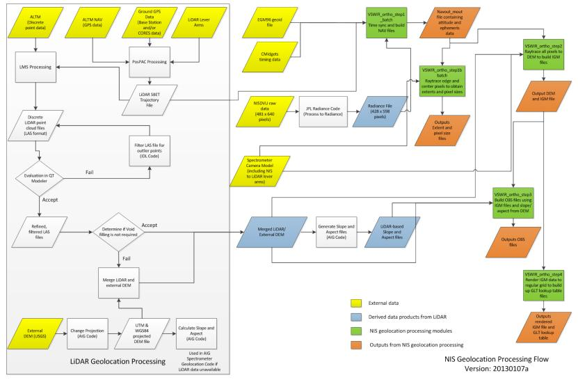
Figure 2. NIS geolocation processing flow
