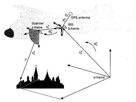
Figure 6. Coordinate transformation from sensor frame to surface frame
