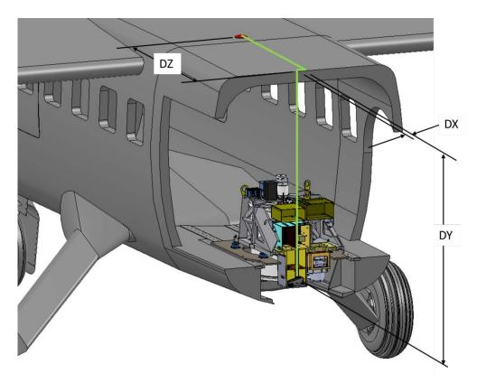
Figure 8. Lever arm calculations for the NISDVU for the configuration flown during May 2012
