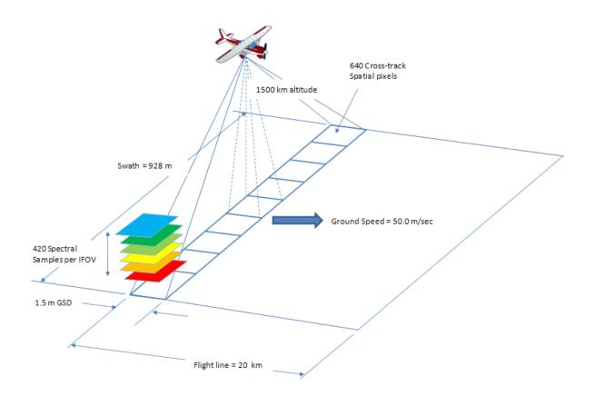
Figure 9. NIS flight geometry
