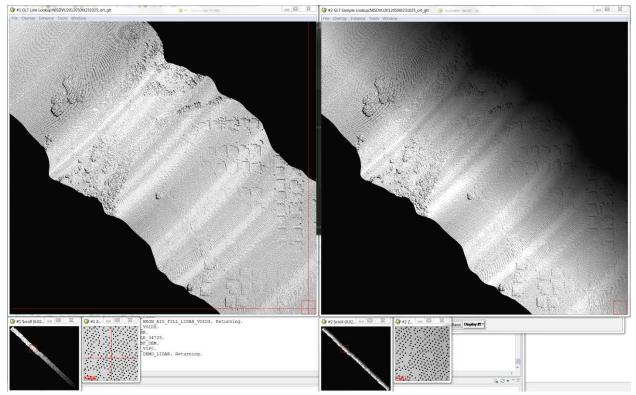
**Figure 1.** Sample GLT Image: The GLT files contain information about which original pixel occupies which output pixel in the final product. The GLT output is sign-coded to indicate whether a certain pixel contains real data (positive) or if it is nearest-neighbor infill pixel (negative).
