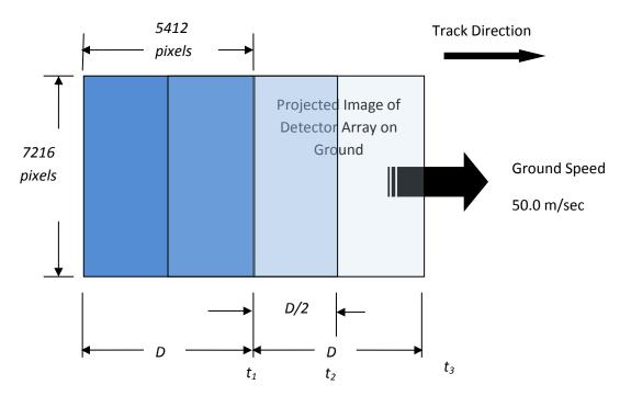
Figure 11. AOP camera scanning approach
