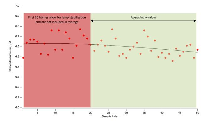
Figure 3. Example of data showing the stabilization of the lamp and the nitrate measurements to be averaged.
