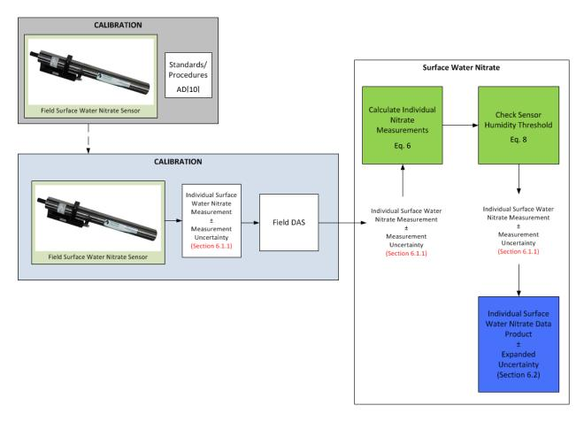
**Figure 3.** Displays the data flow and associated uncertainties of individual measurements of surface water nitrate and associated L1 DPs.
